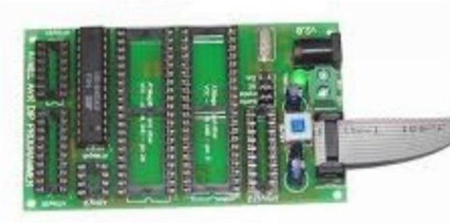
AVR ISP Programming Board Shield ATMEGA8 ATMEGA328P ATTINY2313 ATMEGA32
