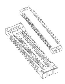
This is space saving type board-to-board connector with 0.4 mm pitch, 0.8 mm between PC boards and 2.0 mm product width.
