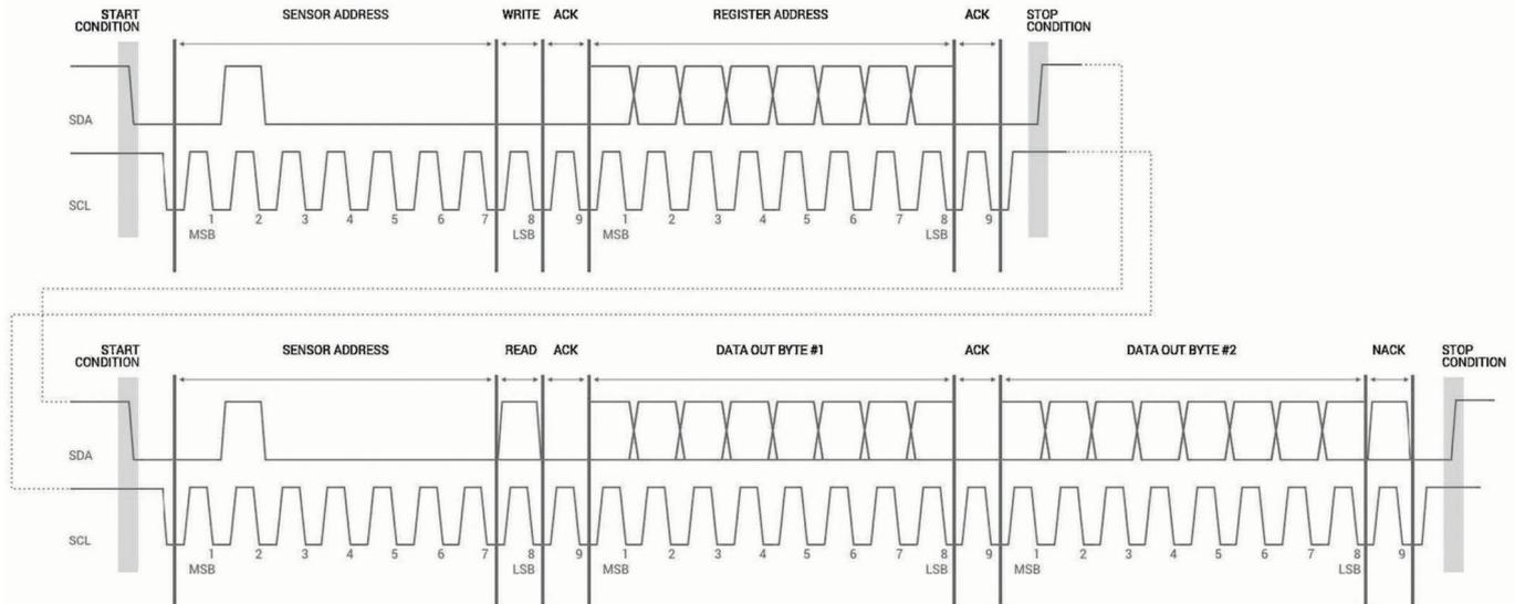
The sensor module has a 7-bit slave address with a default value of 0x62 in hexadecimal notation. The effective 8 bit I2C address is 0xC4 write, 0xC5 read. The device will not respond to a general call.
