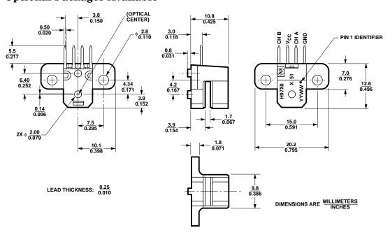
Mounting Option #51 – Screwmount (Baseplane Mounting)
