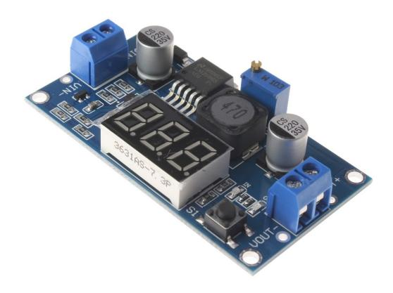
This version of LM2596 DC-DC step-down (buck) power supply module includes the very useful addition of an integrated digital voltage meter. The voltage meter is capable of sensing both input and output supply voltages and can be quickly switched between the two by pressing a voltage selection button on the module...
