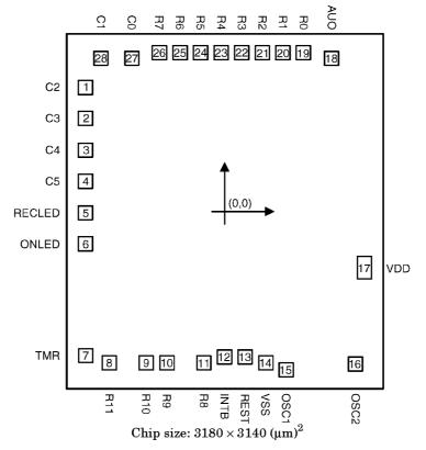
$\ensuremath{^{*}}$  The IC substrate should be connected to VSS in the PCB layout artwork.
