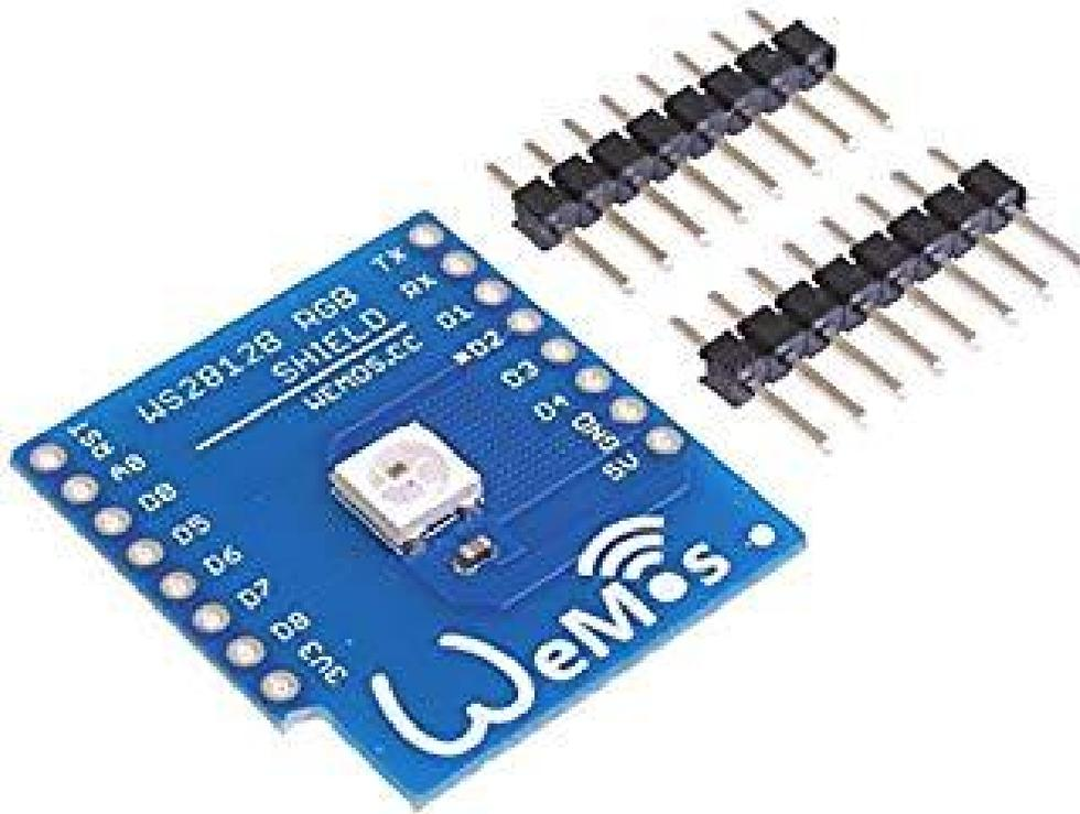
The WeMos WS2812B RGB Shield is a digital full colour (16777216 colour) RGB LED light source. It is specifically designed for the WeMos mini and mini Pro (see item HWEMO0002) ESP8266 based development boards. This shield includes two 8 pin headers (these will require soldering to the module) which will allow it to be easily inserted into the D1 minis headers. To control the LED the shield only requires one digital IO pin (D2).
