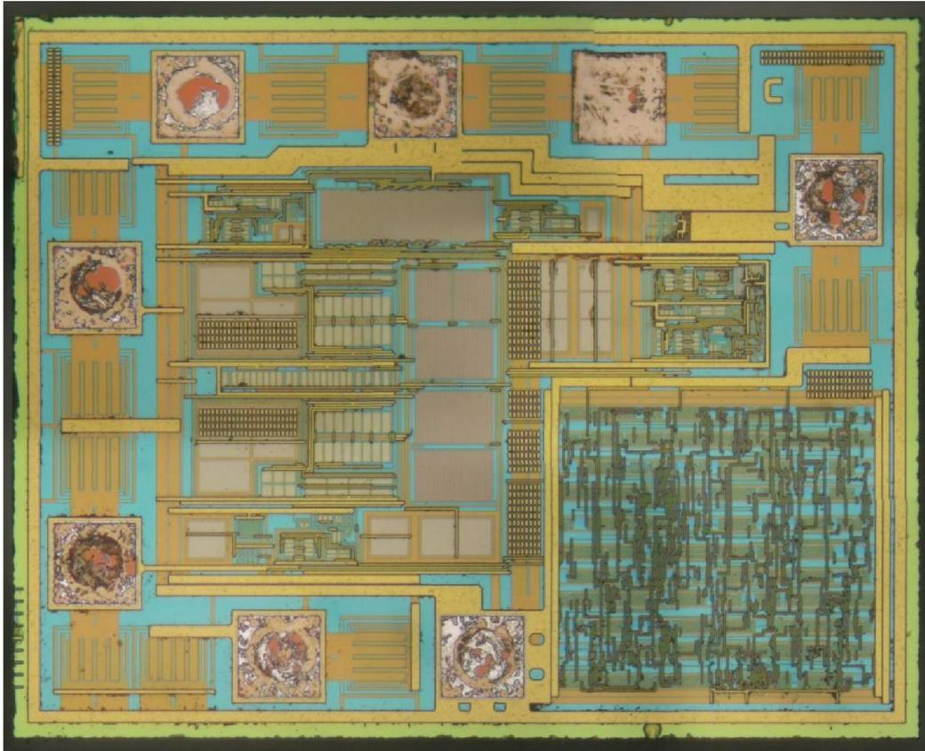
Then there's the chip that does the rest of the processing; let's call this the TT1712. There is a block of logic on the bottom-right, lots of analog circuits in the middle and a label "C" at the top-right. Again, as might be expected, no indication of a manufacturer or even the chip's functionality.
