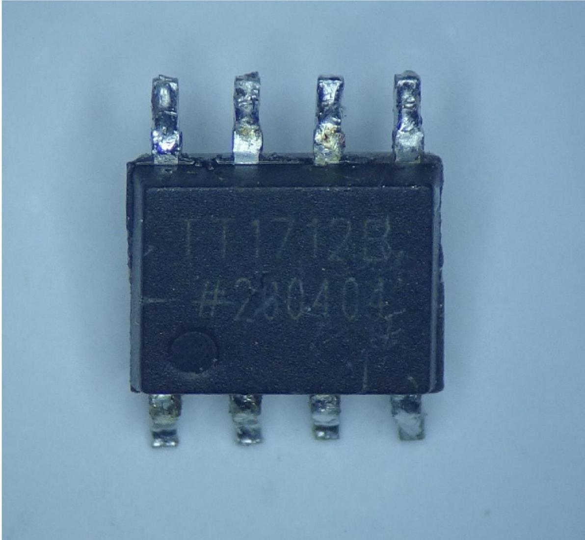
This is the main chip, after removing it from the PCB. The only markings are “TT1712B” and a date code “#200404”. It’s a simple plastic SOIC package with, again, no indication of a manufacturer. On the back it says “1712 1117”, which might indicate the production line or a specific batch.
