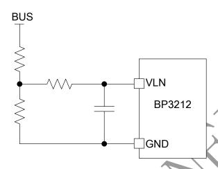
Figure 4. VLN pin application circuit
