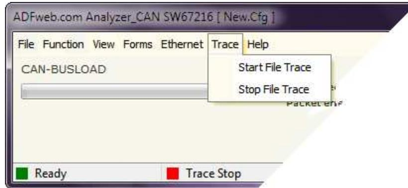
The **Start File Trace** opens a window (Fig. 16) that allows to define the settings of the trace.
