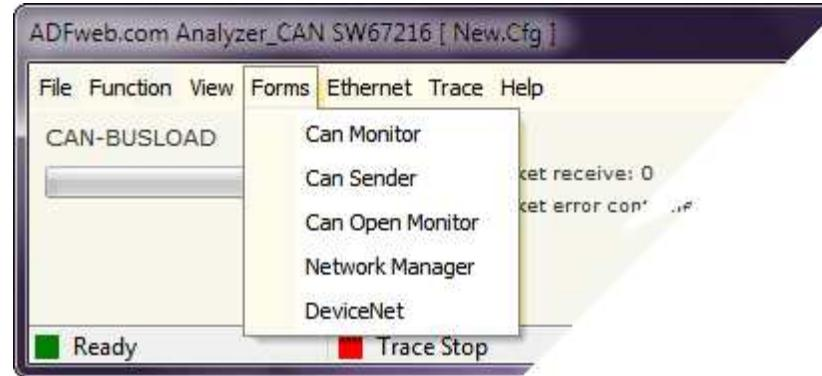
The "**CAN Monitor**" is a window that allows the visualization of the BUS data at the package level.
