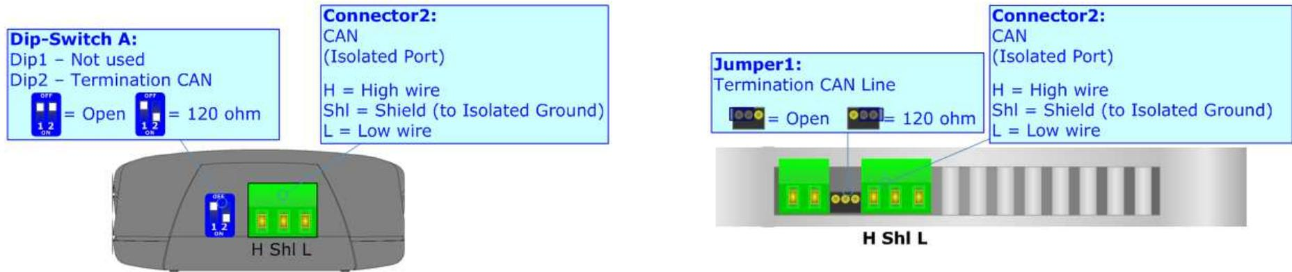
The termination of CAN line, with a 120Ω resistor, in the HD67390-U-D1 is made by putting the “Dip2” of “Dip-Switch A” at “ON” position. The termination of CAN line, with a 120Ω resistor, in the HD67390-E-A1 is made by inserting a jumper like in the figure above.
