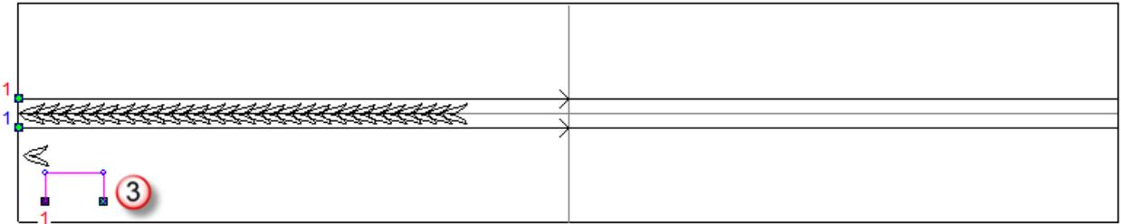
Provided the vectors selected as cross sections contain an equal number of spans, the **Sweep between spans** check box is enabled and selected. The spans and nodes in each subsequent cross section along the drive rails are paired, and the sweep is extruded between them.
