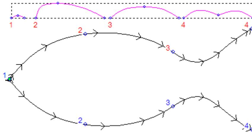
Provided the vectors selected as cross sections contain an equal number of spans, the **Sweep between spans** check box is enabled and selected. The spans and nodes in each subsequent cross section along the drive rails are paired, and the sweep is extruded between them.
