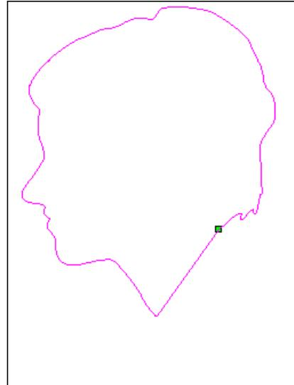
**10** Press the **N** key to enter Node Editing mode. You can see the nodes, spans and control points that make up the polyline you have drawn.
