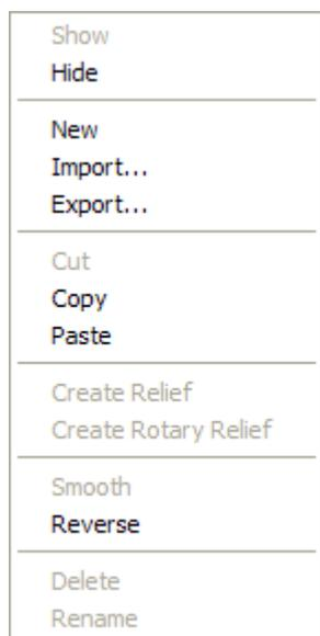
Use this to toggle its visibility, create an empty assembly, import a triangle or surface model, export, copy or paste the root **Assembly**, and reverse the direction of triangles.
