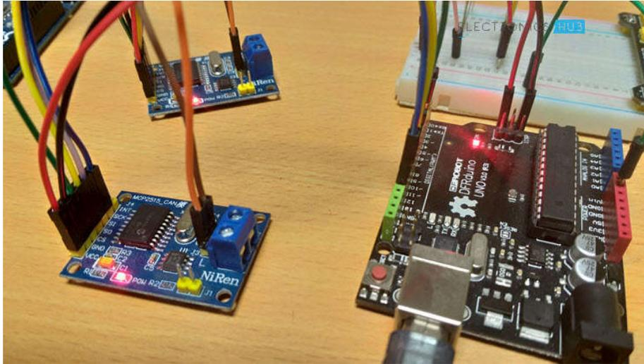
Make two such connections: one pair acts as a transmitter and the other as a receiver. Now for the communication between this transmitter and receiver, connect CANH and CANL pins of each MCP2515 Module.
