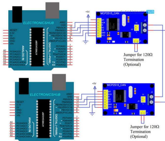
If the pins of the MCP2515 Module are not clear, the following image might be useful.
