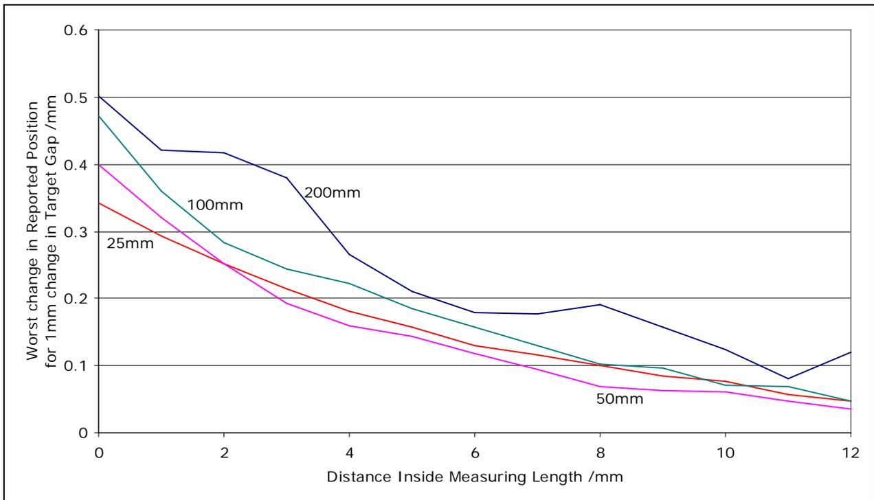
Figure 17 Effect of 1mm change in Target Gap from Nominal
