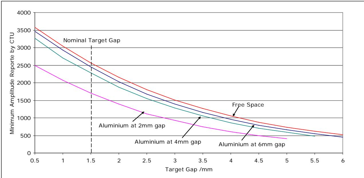
Figure 28 Reported Amplitude with an Aluminium sheet behind 50mm sensor
