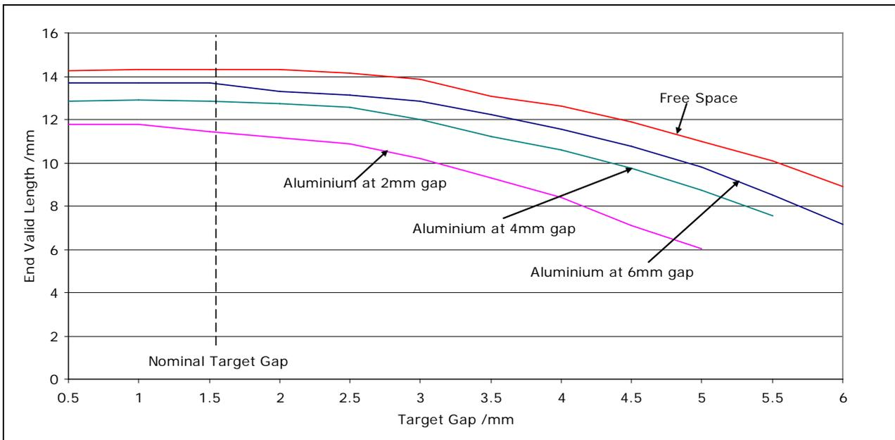
Figure 29 End Valid Length with an Aluminium sheet behind 50mm sensor
