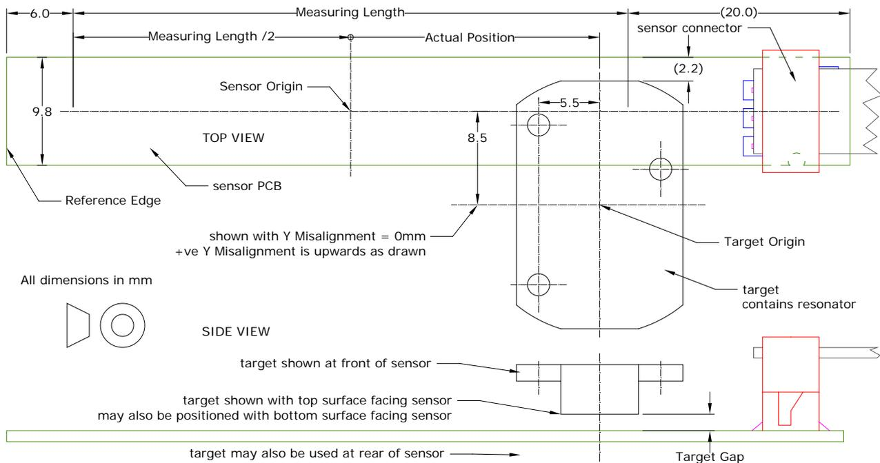
Figure 3 assembled sensor shown with target part number 013-1005
