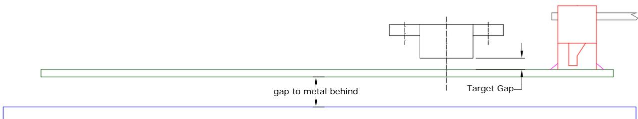
Figure 27 metal behind sensor
