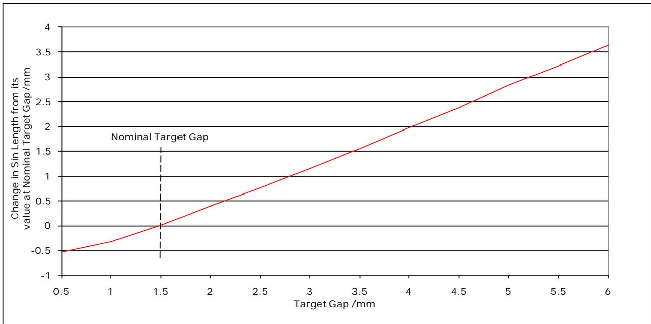
**Figure 16 Sin Length dependence on Target Gap**
