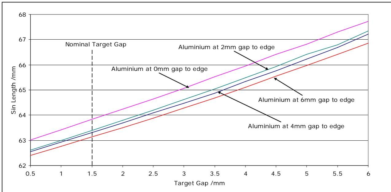
Figure 36 Sin Length with an Aluminium sheet at edge of 50mm sensor
