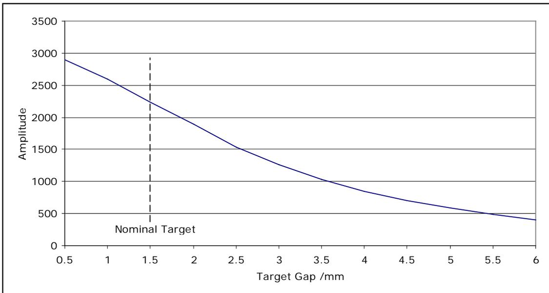
Figure 26 Amplitude reported by CTU versus Target Gap
