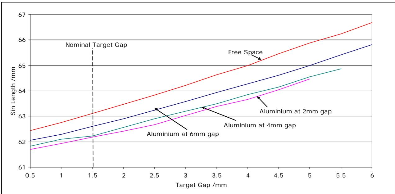
Figure 31 Sin Length with an Aluminium sheet behind 50mm sensor
