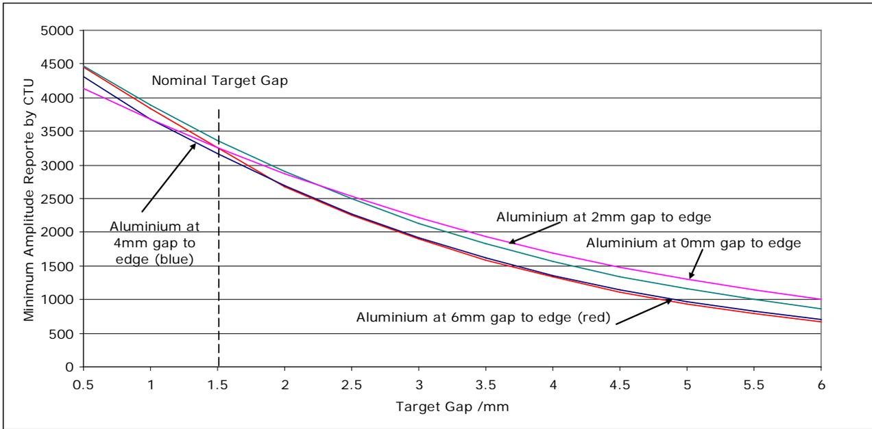
Figure 33 Reported Amplitude with an Aluminium sheet at edge of 50mm sensor
