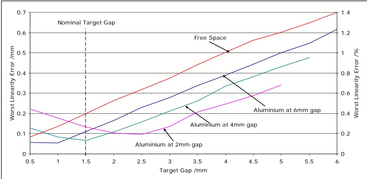
Figure 30 Linearity Error with an Aluminium sheet behind 50mm sensor
