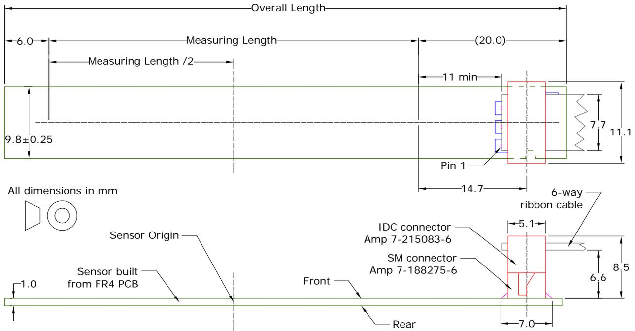
Figure 4 assembled sensor, shown with connector 013-6001 attached
