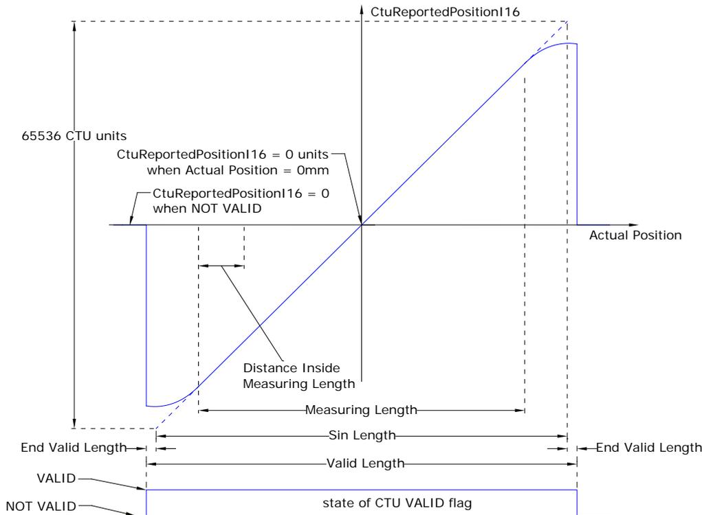
**Figure 5 CTU outputs versus position**
