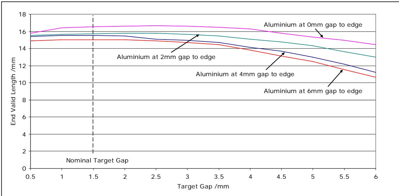
Figure 34 End Valid Length with an Aluminium sheet at edge of 50mm sensor
