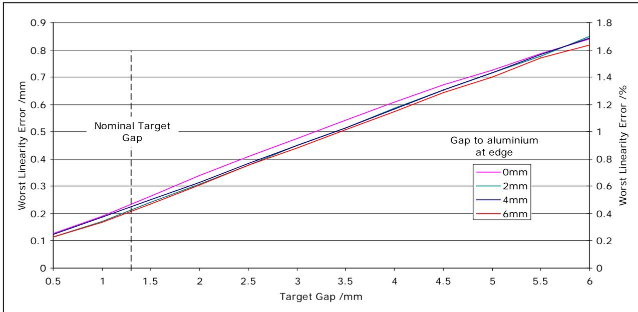
Figure 35 Linearity Error with an Aluminium sheet at edge of 50mm sensor
