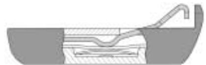
**Card detection switches** - As a manufacturer of switches as well as connectors, we have been able to integrate high performance dome switches into many of our connectors. These are variants of switch products which are already in high volume production as standalone components.
