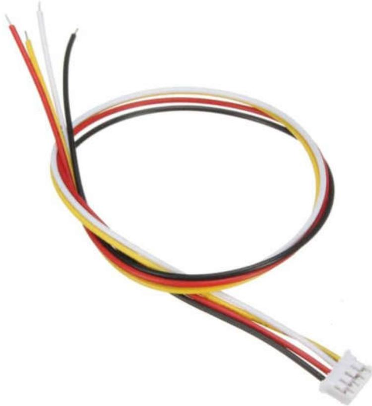
JST connector set commonly used in the robotics and R/C hobby industry. Each set includes a female connector with 29cm (11.4") of red/black/yellow 26AWG connection wire along with a male PCB mount connector.
