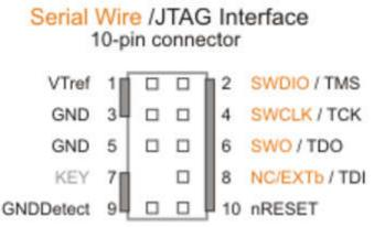
Many debugger tools (such as Segger J-Link) will typically only provide the 20-pin ARM connector(0.1" pin spacing) as an output. This connector has many of the same pins as the 10-pin version, but also provides other non essential functions for JTAG or SWD MCU devices. So you may have to do a translation from the 20-pin connector to the 10-pin connector using an adaptor. The following image shows the 20-pin connector pin out:
