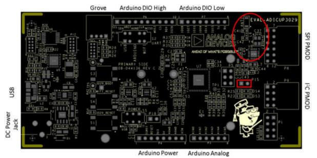
The ADuCM3029 communicates to the EM9304 using the SPI2 bus from the ADuCM3029. So users will need to send BLE commands and data over SPI2 bus. Library functions and API calls have been specifically designed to be used with the ADuCM3029 and EM9304 using SPI2 bus, so the user will only need to configure and send data over BLE.
