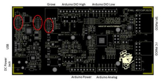
All three connectors used are based off the 10-pin ARM Cortex standard pin out(0.05" pin spacing). That pin out is common to both JTAG and SWD debug modes and is depicted in the following image.
