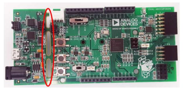
You'll be left with two separate boards, the left hand side will be the "Debugger board" and the right hand side will be the "ADICUP3029 node board"
