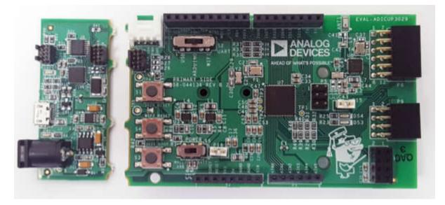
Once apart, the user can use the debugger board, and a standard 10-pin ARM JTAG/SWD ribbon cable to connect to the ADICUP3029 node board. And using the CrossCore Embedded Studio IDE, program an updated or new application into the ADICUP3029 IoT node.
