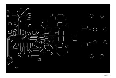
FIGURE 11. Reference PCB Bottom Layer
