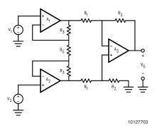
FIGURE 5. Feedback instrumentation Amplifier Schematic
