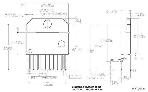
Non-Isolated TO-220 15-Lead Package Order Number LM4652TA **NS Package Number TA15A**
