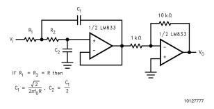
FIGURE 6. Pre-amplifier Stage with Low Pass Filter
