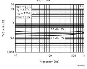
THD+N vs. Frequency vs. Bandwidth  $R_L = 8\Omega$
