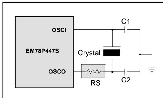
Fig. 4-10 Crystal/Resonator Circuit
