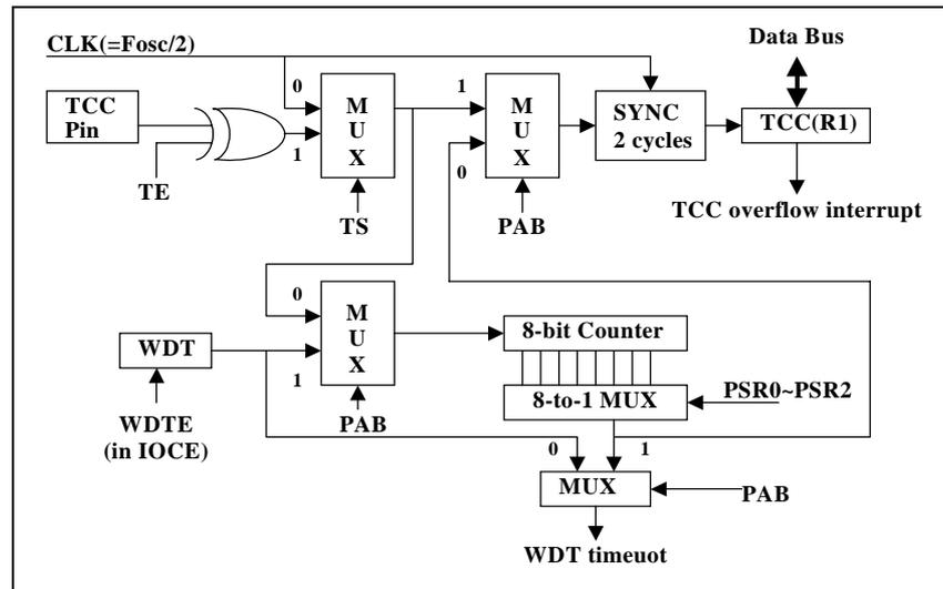
Fig. 4-5 TCC and WDT Block Diagram
