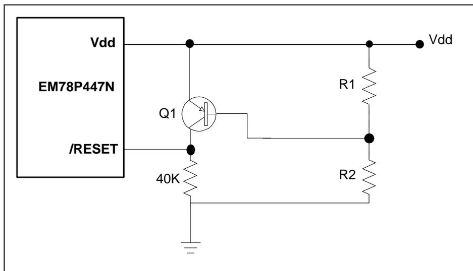
Fig.4-14 Residue Voltage Protection Circuit 2
