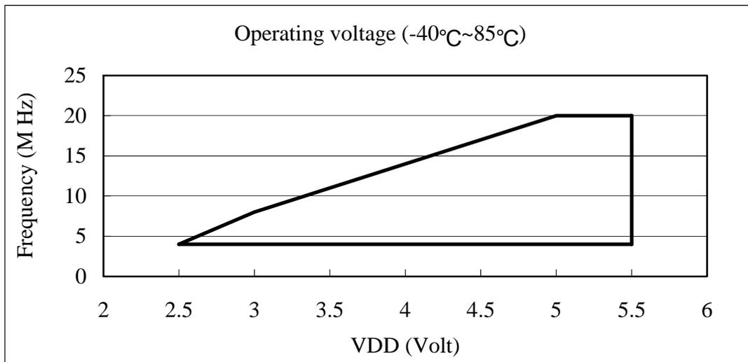
Fig. 6-18 Operating Voltage In Temperature Range from  $-40\text{ }^{\circ}\text{C}$  to  $85\text{ }^{\circ}\text{C}$
