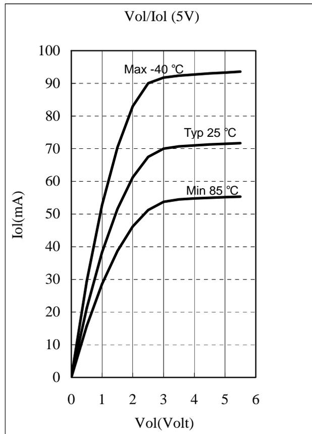
Fig. 6-7 Port 7 Vol vs. Iol, VDD=5V
