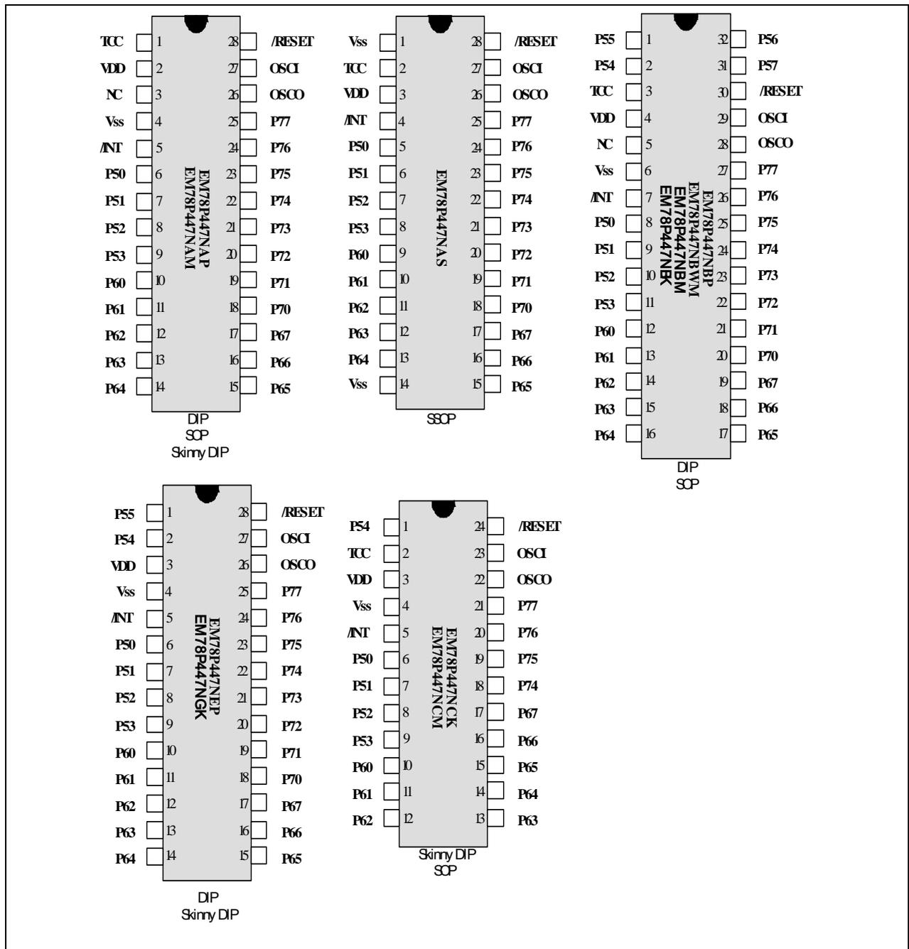
Fig. 3-1 Pin Assignment
