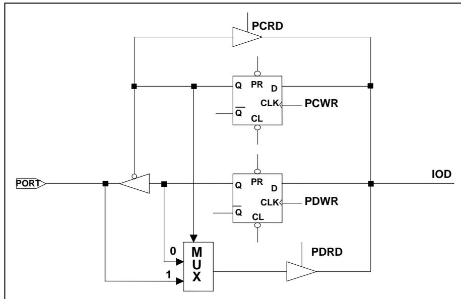
Fig. 4-6 (a) I/O Port and I/O Control Register Circuit
