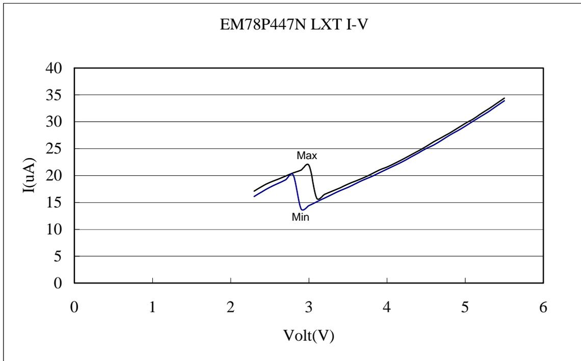
Fig. 6-20 EM78P447N I-V Curve Operating at 32.768 kHz
