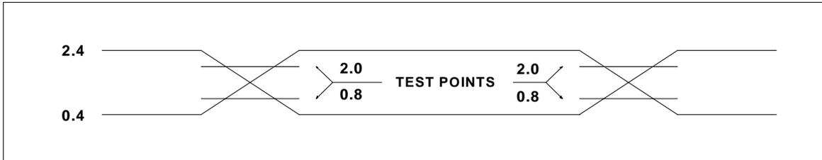
AC Testing : Input is driven at 2.4V for logic "1",and 0.4V for logic "0".Timing measurements are made at 2.0V for logic "1",and 0.8V for logic "0".
