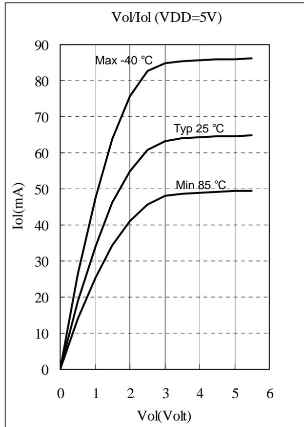
Fig. 6-5 Port 5, and Port 6 Vol vs, Iol, VDD=5V
