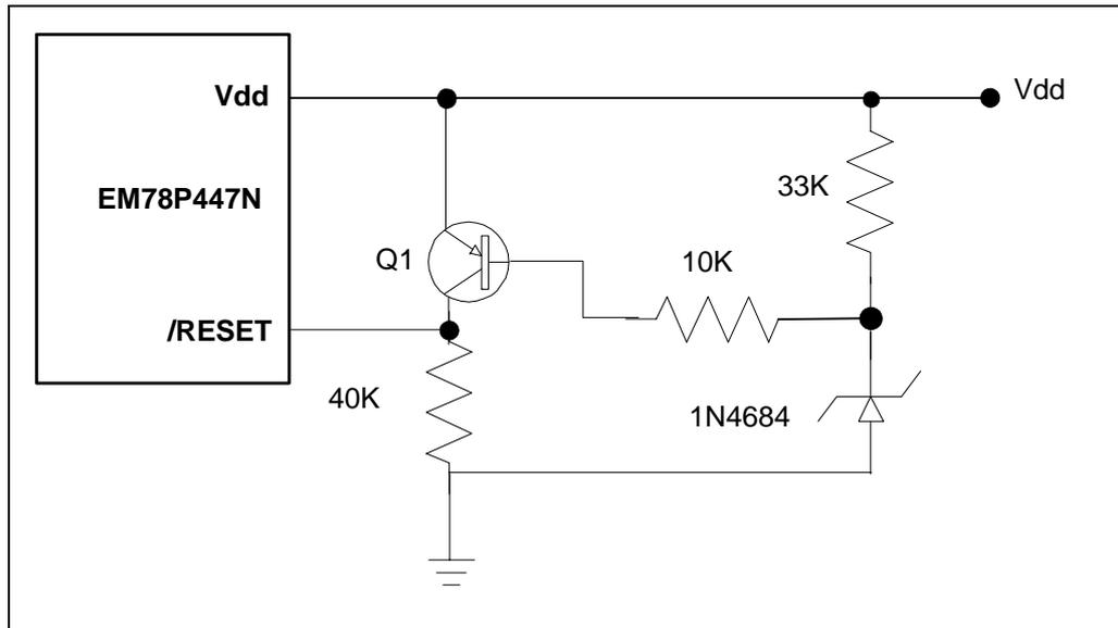
Fig.4-13 Residue Voltage Protection Circuit 1
