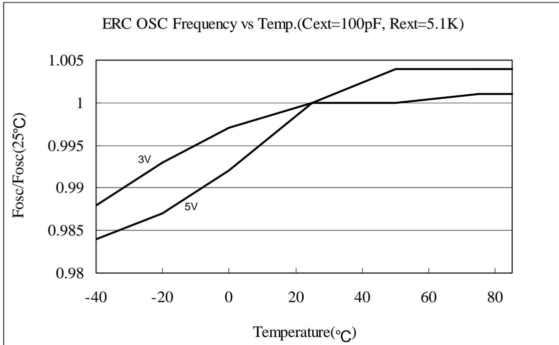
Fig. 6-11 Typical RC OSC Frequency vs. Temperature ( R and C are ideal component )
