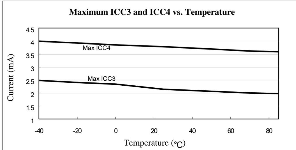
Fig. 6-15 Maximum Operating Current ( ICC3 and ICC4 ) vs. Temperature
