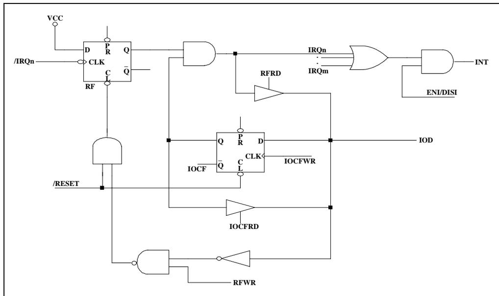
Fig. 4-8 Interrupt Input Circuit
