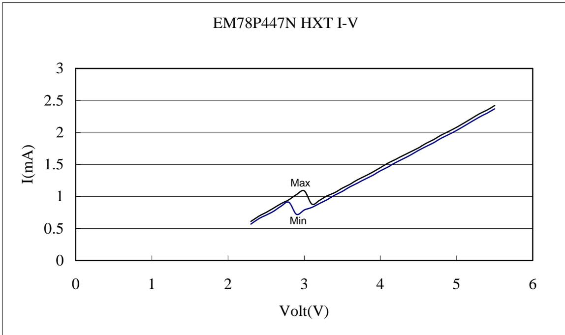
Fig. 6-19 EM78P447N I-V Curve Operating at 4 MHz
