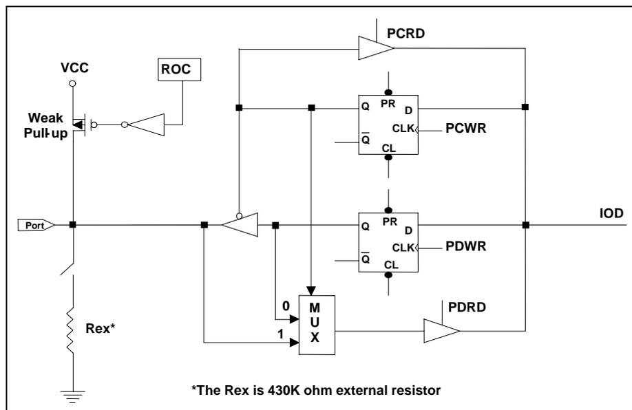
Fig.4-6 (b) I/O Port with R-Option (P70, P71) Circuit
