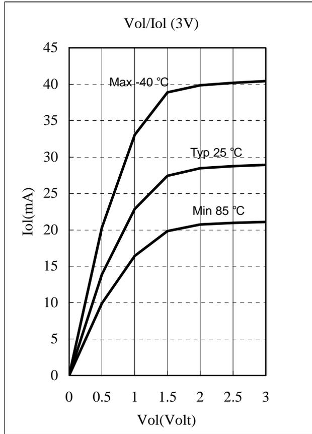
Fig. 6-8 Port 7 Vol vs. IoI, VDD=3V
