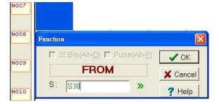
Enter "S30", press "OK", and the S30 component of the FROM function will appear in the program area. Single-click behind the contact A component, enter the reference number "X3"; or immediately input "AX3", as shown in the window below:
