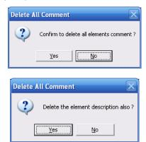
After you confirm the clear all operation, all descriptions and annotations in the project files will be deleted from the storage disk, and if you are connected to the PLC, then the following screen will appear, which represents that the annotations and descriptions in the PLC will also be deleted:
