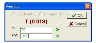
Enter "T0" into the [T] field; enter "1000" into the [PV] field, and you have completed the settings for a set period timer:
