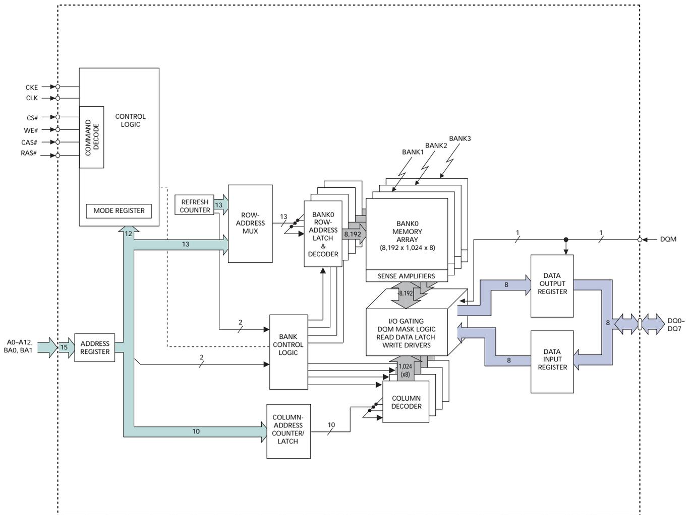
Figure 3: 16 Meg x 16 SDRAM Functional Block Diagram
