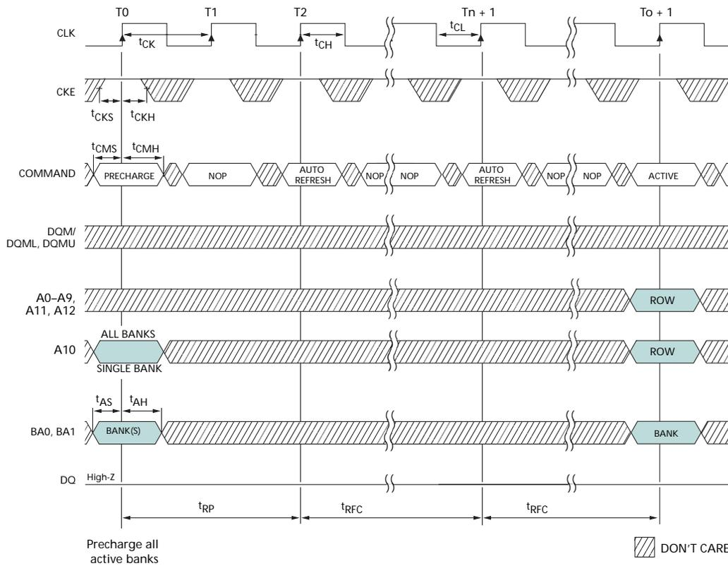
Notes: 1. t<sub>RFC</sub> must not be interrupted by any executable command; COMMAND INHIBIT or NOP must be applied on each positive edge during t<sub>RFC</sub>.
