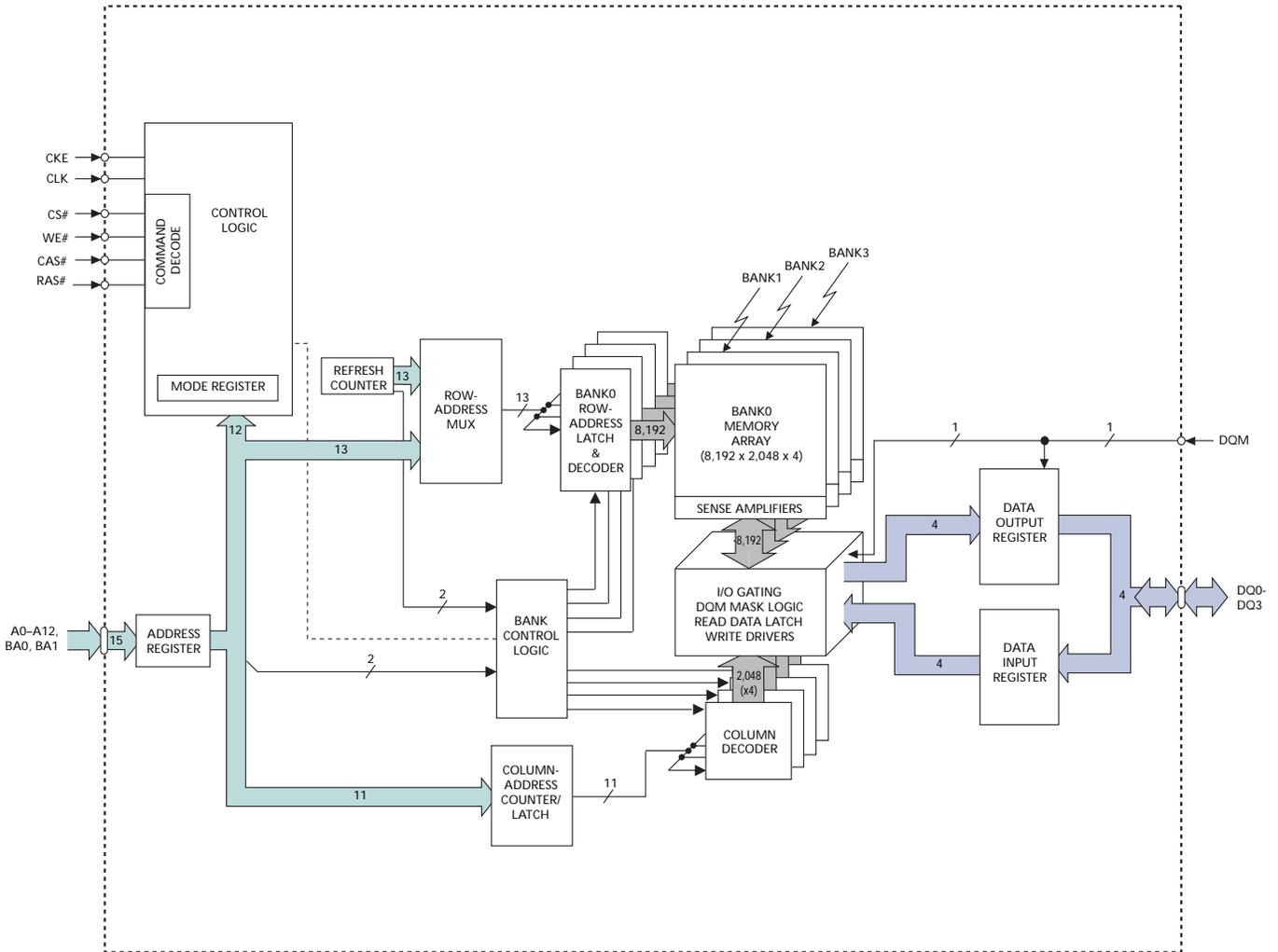
Figure 2: 32 Meg x 8 SDRAM Functional Block Diagram
