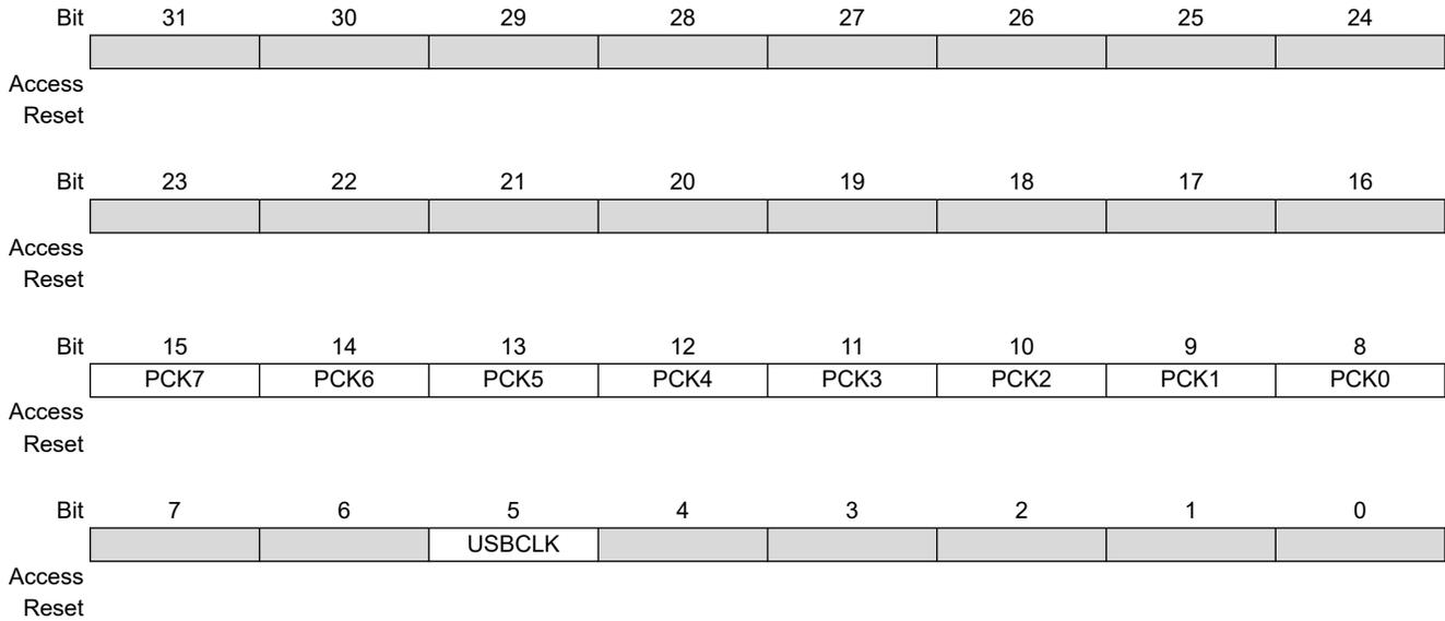
**Bits 8, 9, 10, 11, 12, 13, 14, 15 – PCK** Programmable Clock x Output Enable
