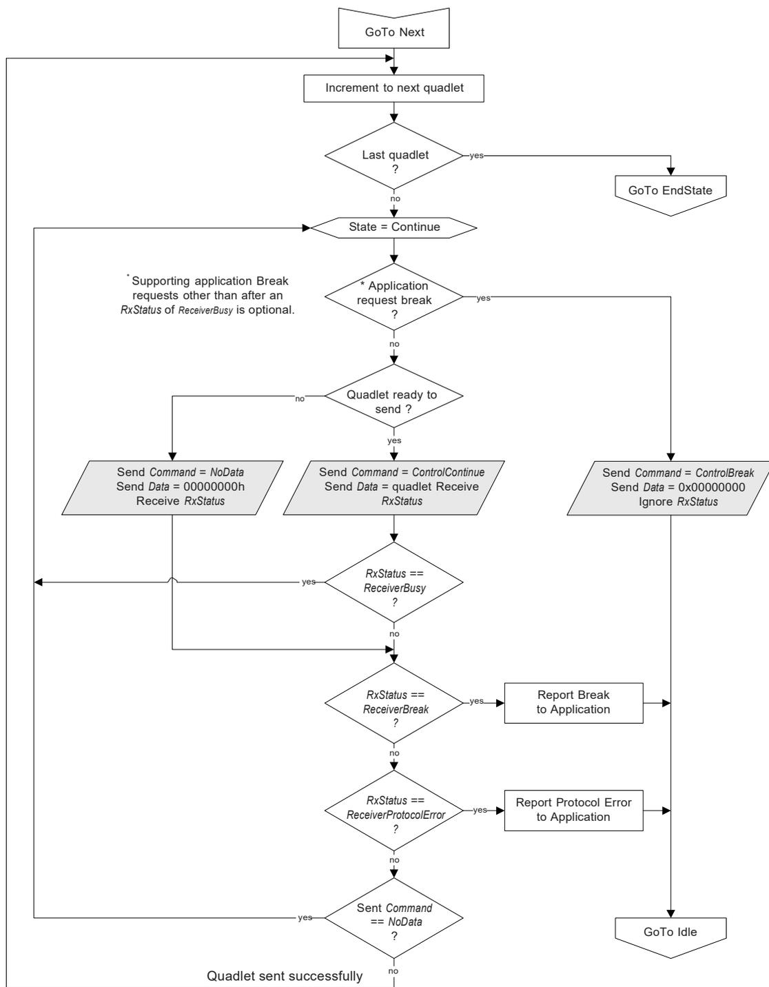
**Figure 48-8. Control Packet Tx Device Protocol: End**
