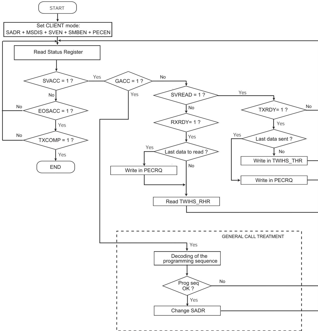
**Figure 43-45. Read Write Flowchart in Client Mode with SMBus PEC and Alternative Command Mode**
