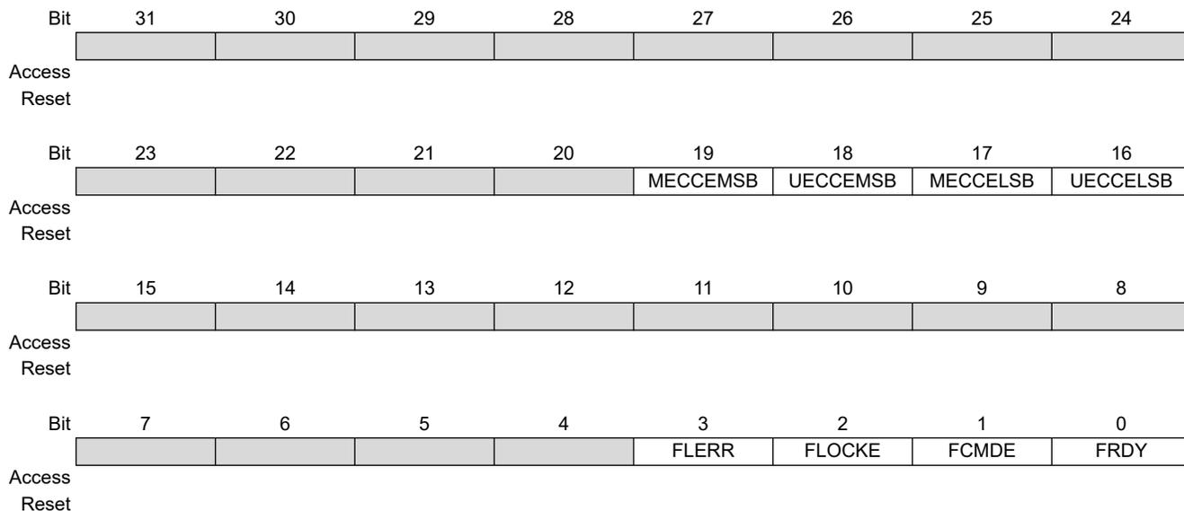
**Bit 19 – MECC EMSB** Multiple ECC Error on MSB Part of the Memory Flash Data Bus (cleared on read)
