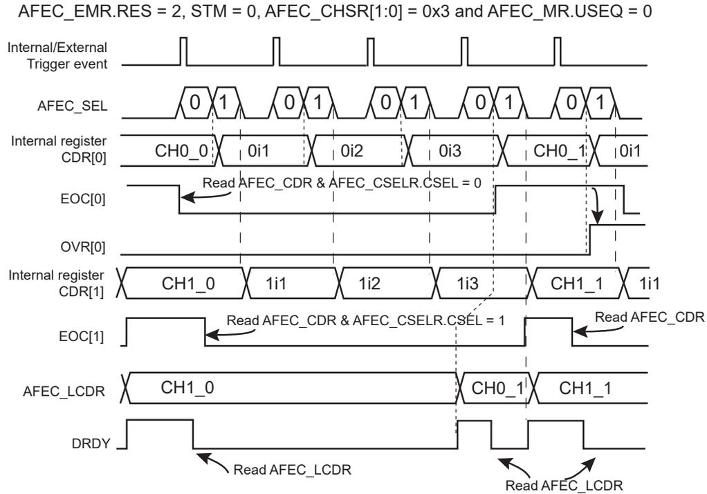
If AFEC\_EMR.STM is set and AFEC\_MR.USEQ is cleared, the sequence to be converted, defined in the AFEC\_CHSR, is automatically repeated n times, where n corresponds to the oversampling ratio defined AFEC\_EMR.RES. As a result, only one trigger is required to get the result of the averaging function as shown in the figure below.
