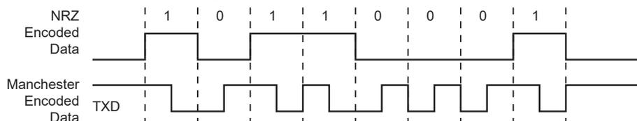
The Manchester encoded character can also be encapsulated by adding both a configurable preamble and a start frame delimiter pattern. Depending on the configuration, the preamble is a training sequence, composed of a predefined pattern with a programmable length from 1 to 15 bit times. If the preamble length is set to '0', the
