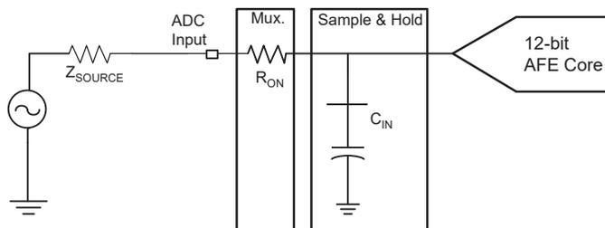
During the tracking phase, the AFE tracks the input signal during the tracking time shown below:
