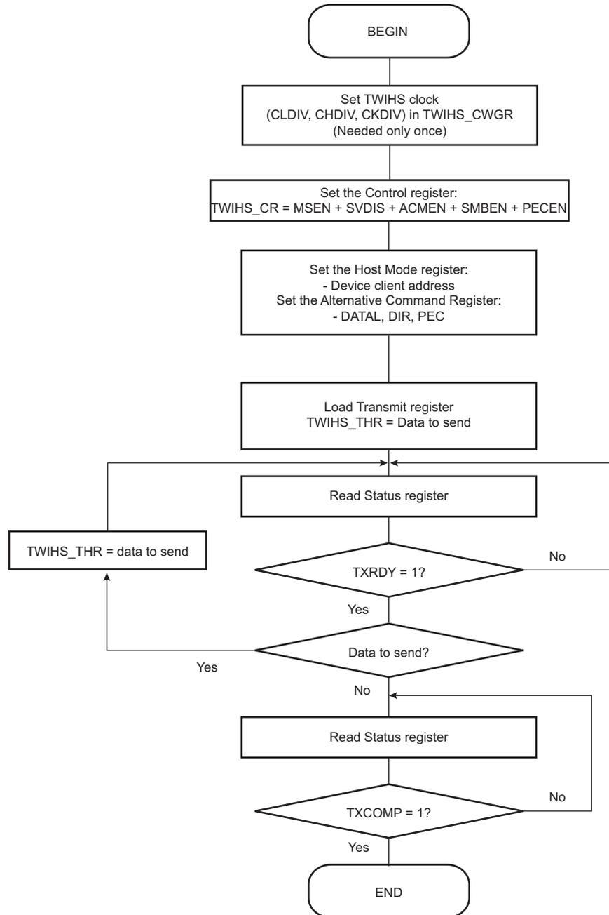
**Figure 43-19. TWIHS Write Operation with Multiple Data Bytes and Read Operation with Multiple Data Bytes (Sr)**
