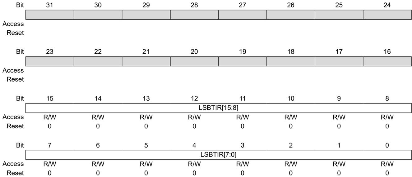
**Bits 15:0 – LSBTIR[15:0]** Lower Significant Bits of Timer Increment Register
