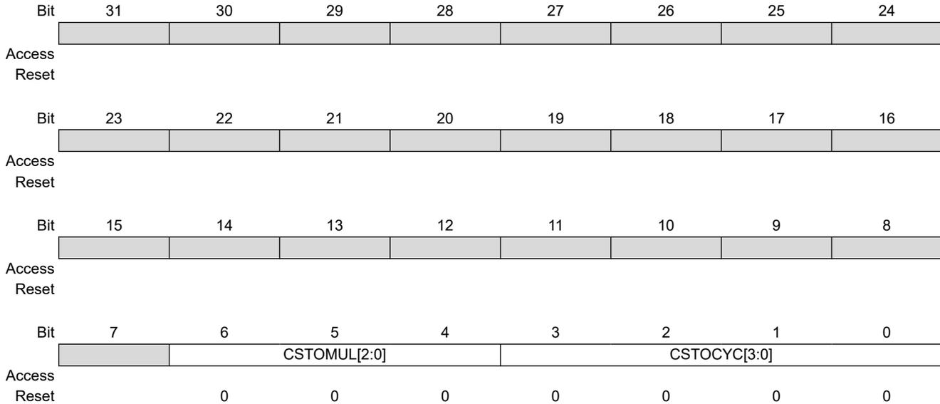
**Bits 6:4 – CSTOMUL[2:0]** Completion Signal Timeout Multiplier
