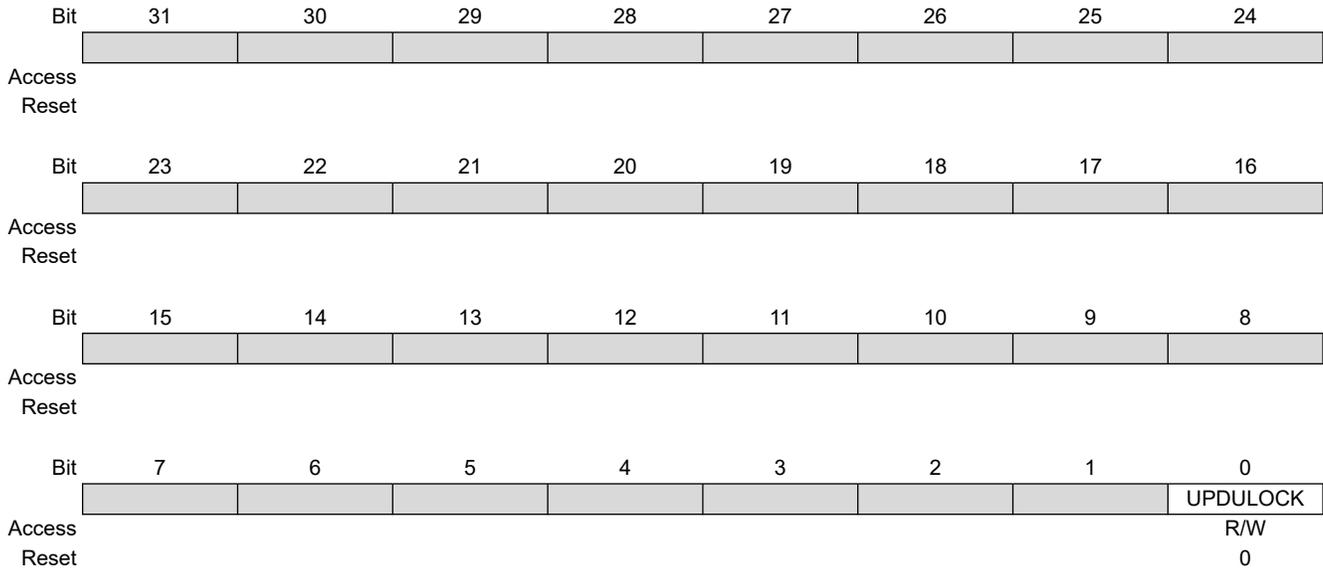
**Bit 0 – UPDULOCK** Synchronous Channels Update Unlock
