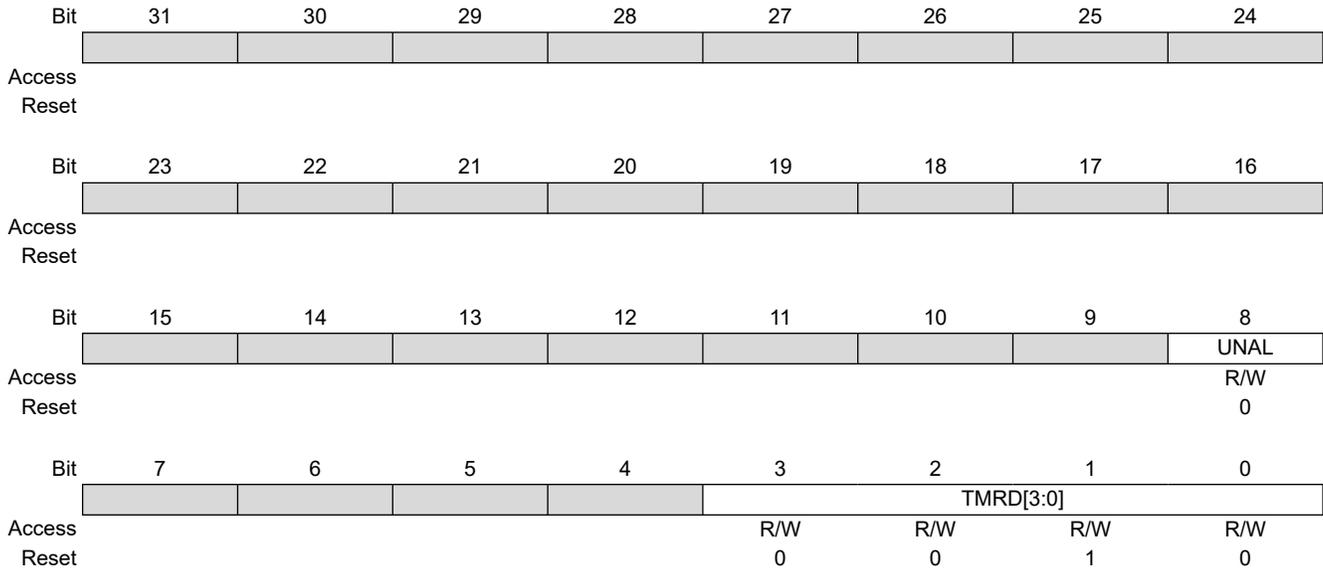
**Bit 8 – UNAL** Support Unaligned Access
