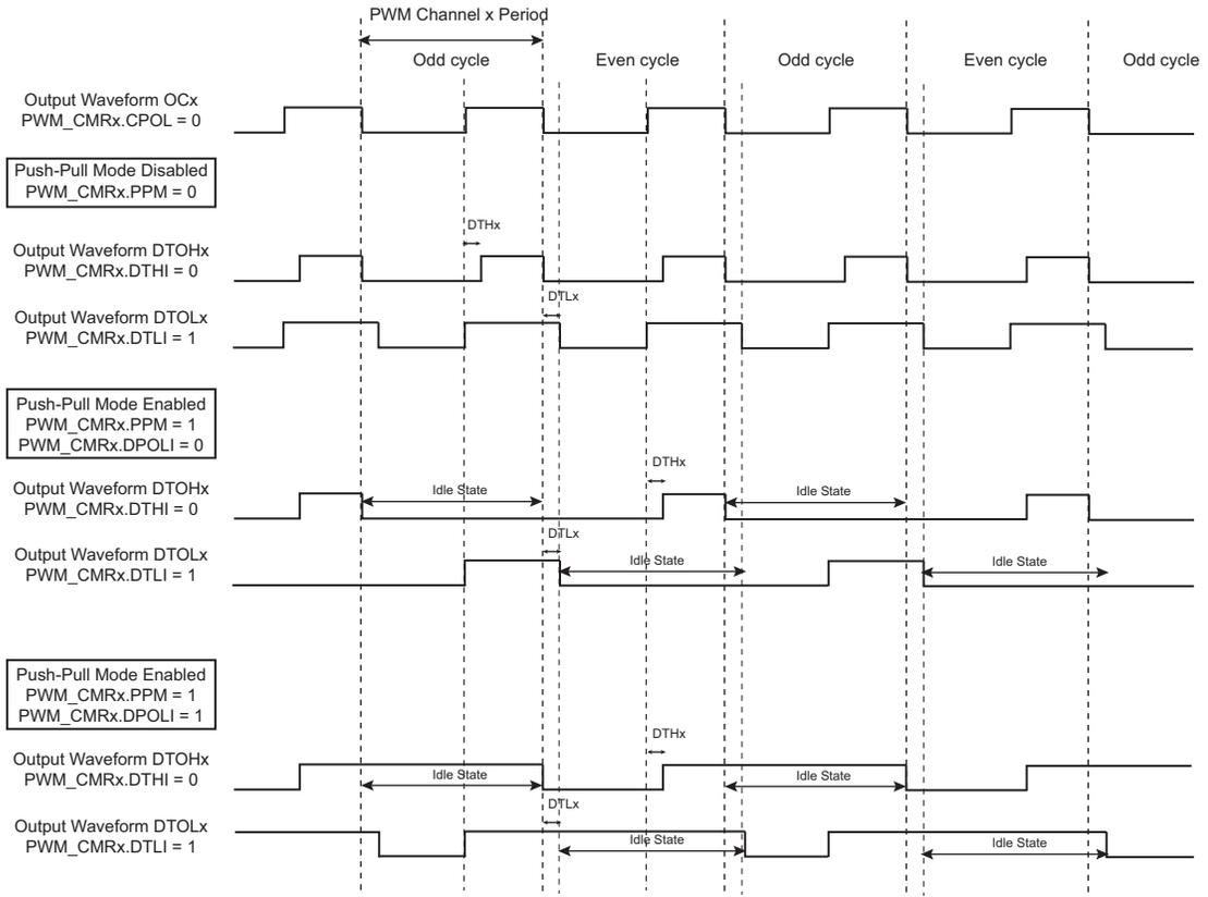
**Figure 51-11. PWM Push-Pull Waveforms: Left-Aligned Mode**
