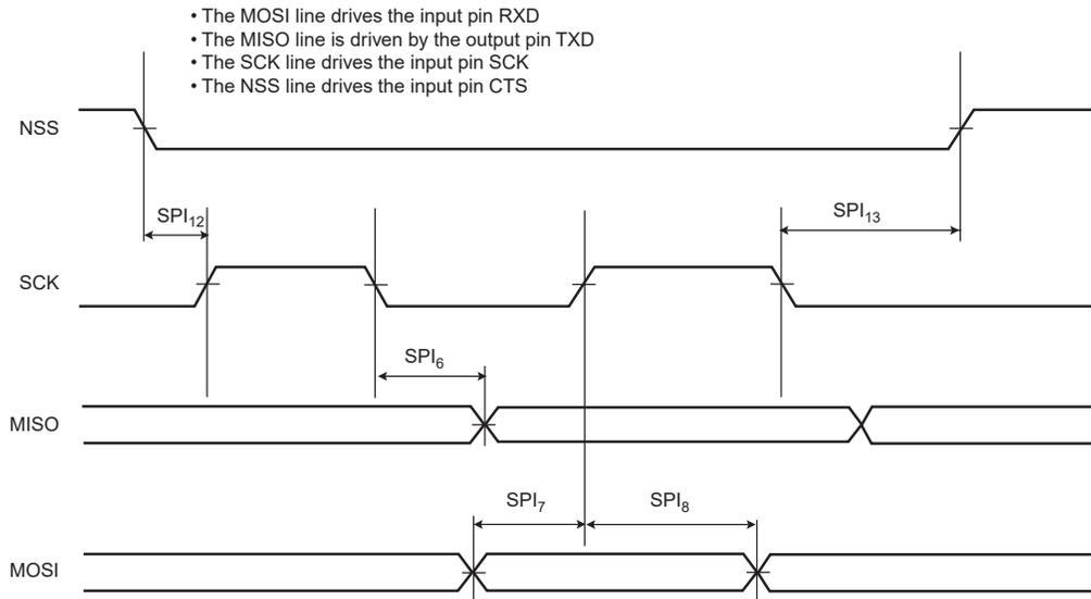
**Figure 59-26. USART SPI Client Mode (Mode 0 or 3)**
