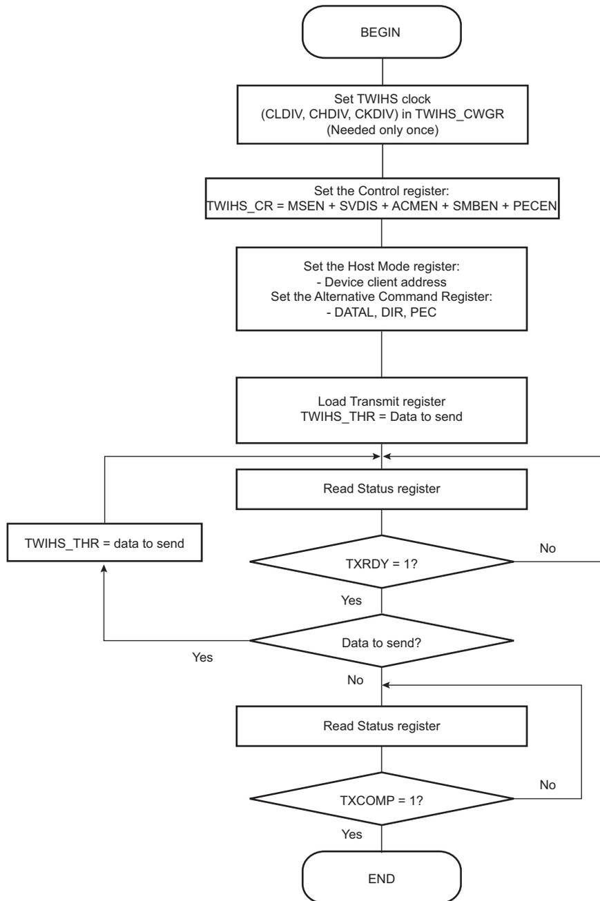
**Figure 43-21. TWIHS Read Operation with Single Data Byte without Internal Address**
