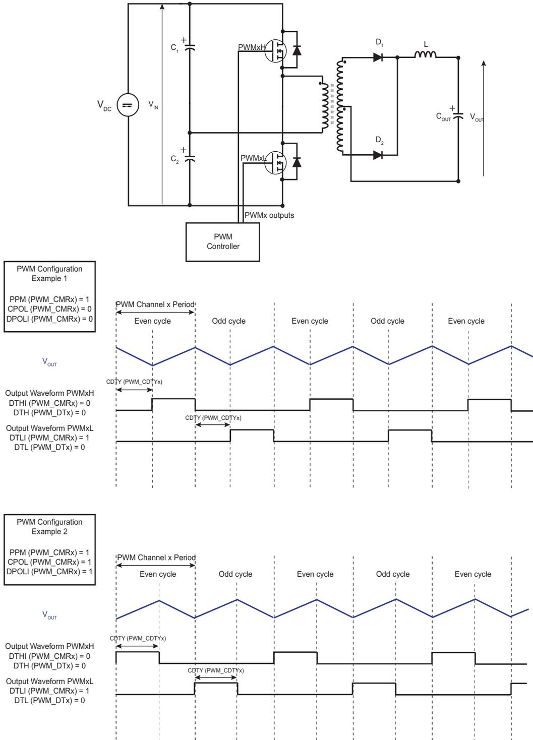
**Figure 51-14. Half-Bridge Converter Application: Feedback Regulation**
