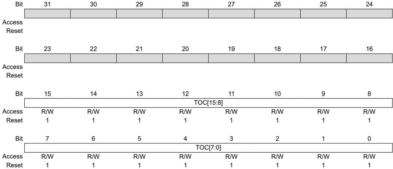
**Bits 15:0 – TOC[15:0]** Timeout Counter (cleared on write)
