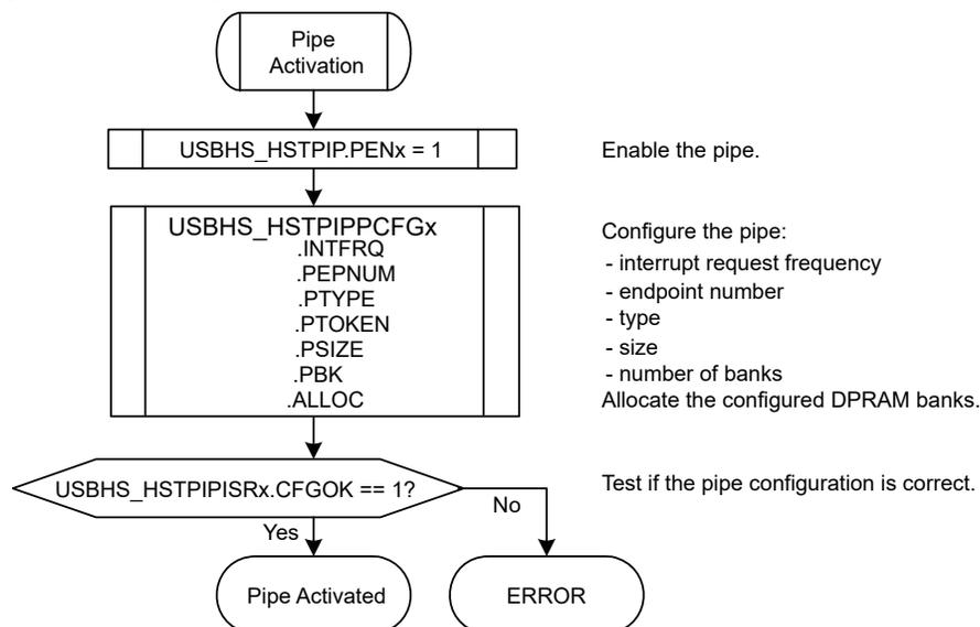
As long as the pipe is not correctly configured (USBHS\_HSTPIPISRx.CFGOK = 0), the controller cannot send packets to the device through this pipe.
