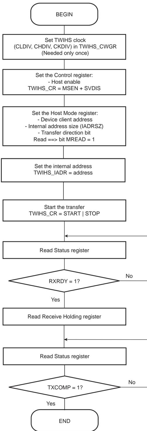
**Figure 43-23. TWIHS Read Operation with Multiple Data Bytes with or without Internal Address**
