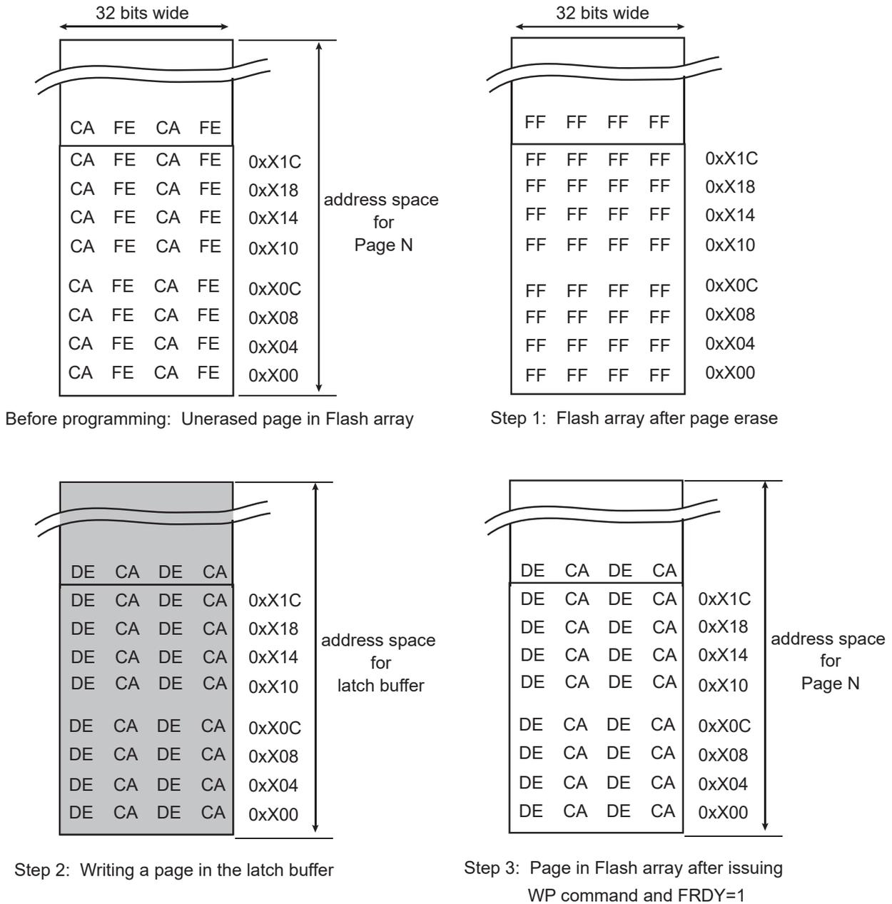
**Figure 22-11. Programming Bytes in the Flash**
