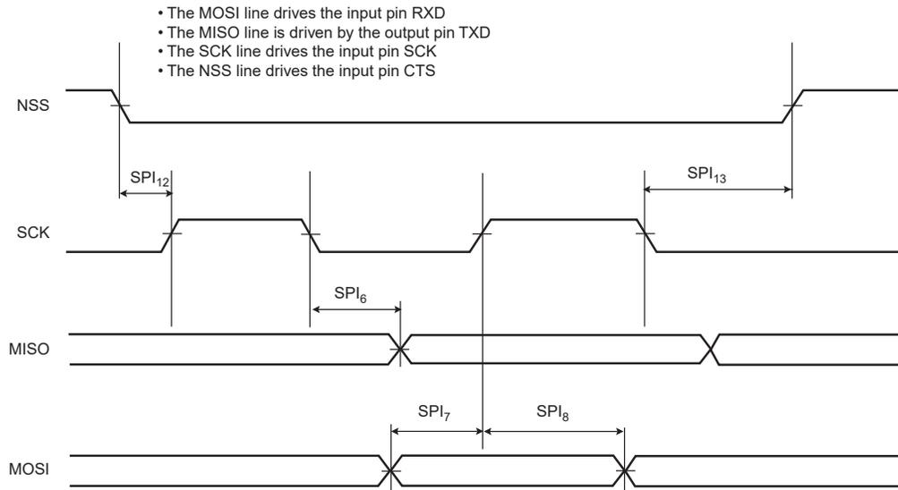
**Figure 58-28. USART SPI Client Mode (Mode 0 or 3)**
