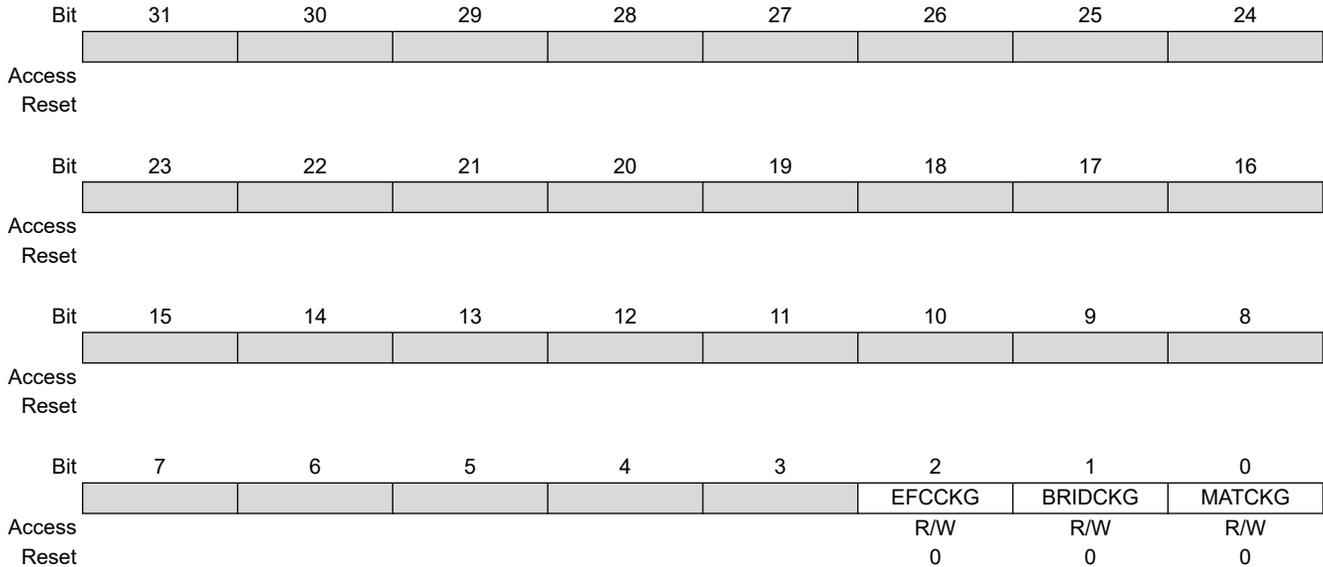
**Bit 2 – EFCCKG** EFC Dynamic Clock Gating Enable
