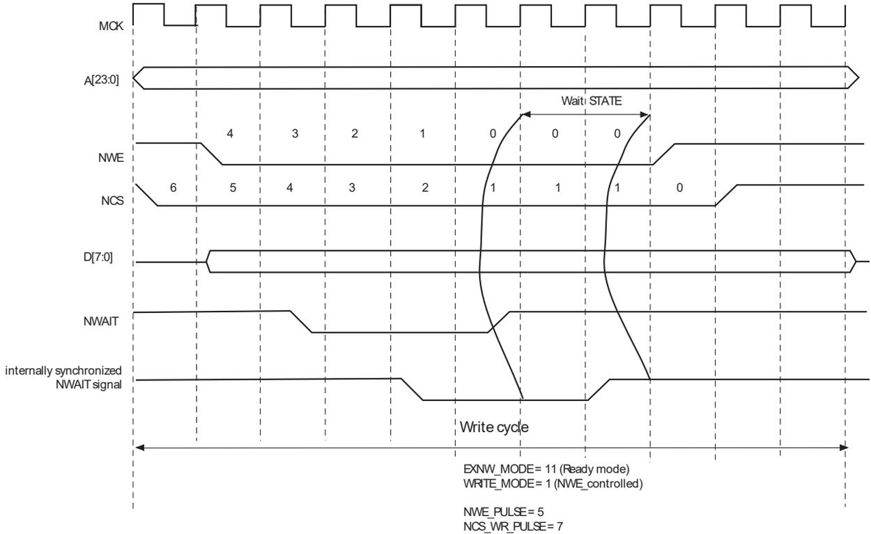
**Figure 35-30. NWAIT Assertion in Read Access: Ready Mode (SMC\_MODE.EXNW\_MODE = 11)**
