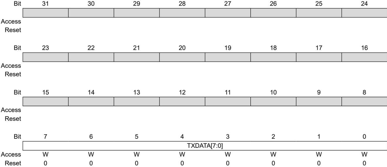
**Bits 7:0 – TXDATA[7:0]** Host or Client Transmit Holding Data
