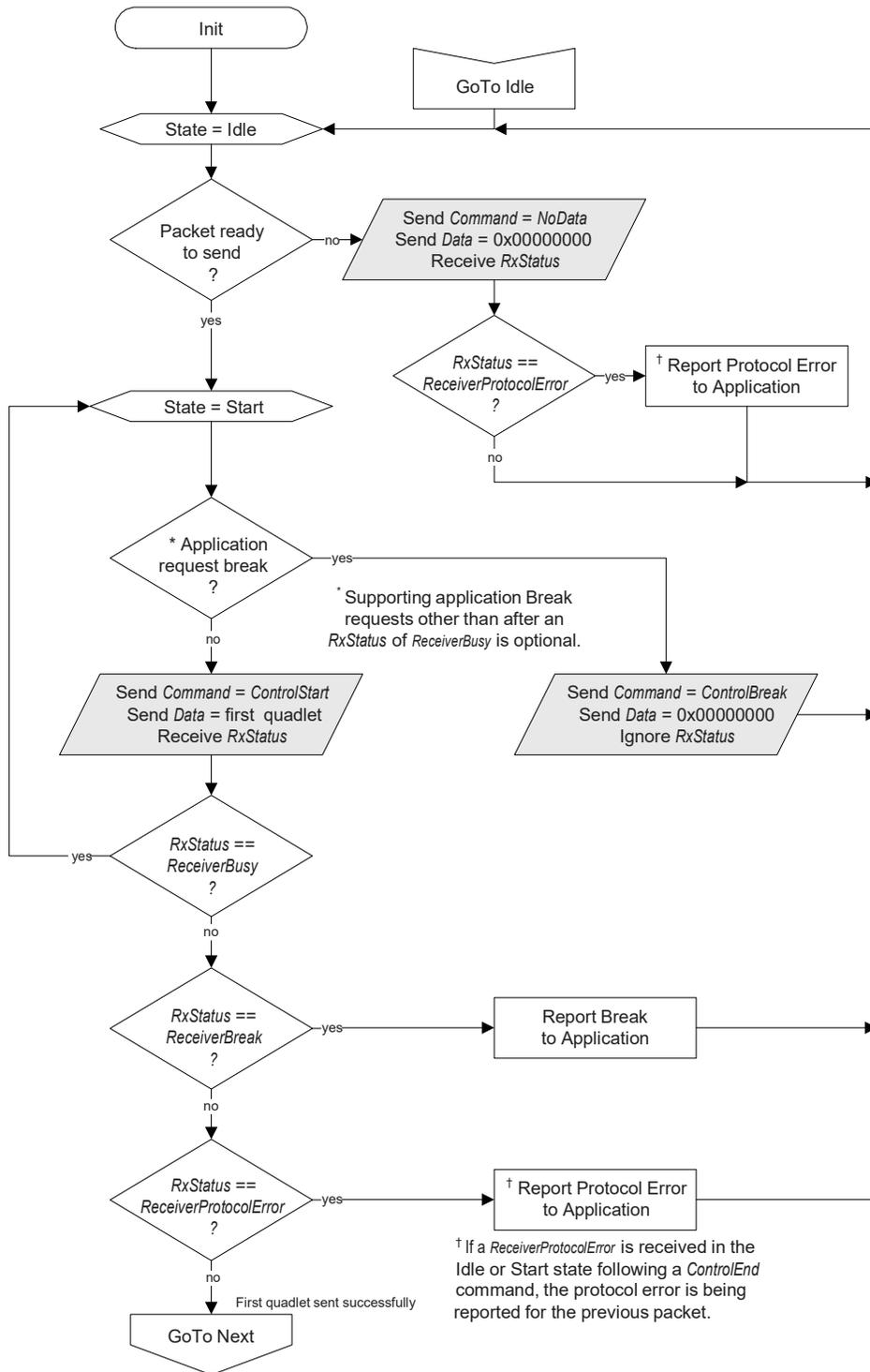
**Figure 48-7. Control Packet Tx Device Protocol: Middle**
