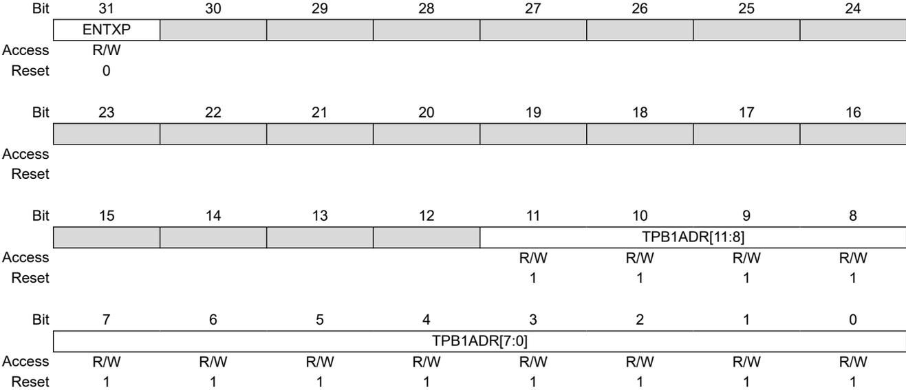
**Bit 31 – ENTXP** Enable TX Partial Store and Forward Operation
