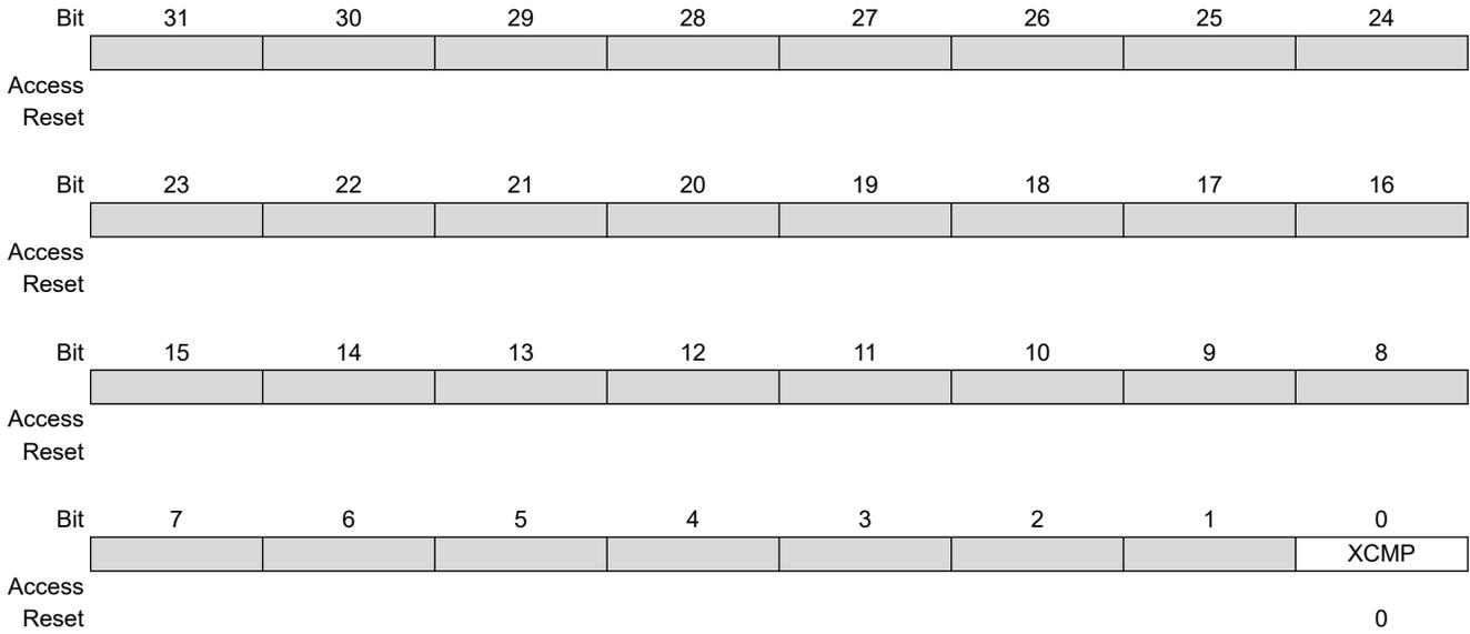
**Bit 0 – XCMP** Transfer Complete (Write 0 to Clear)
