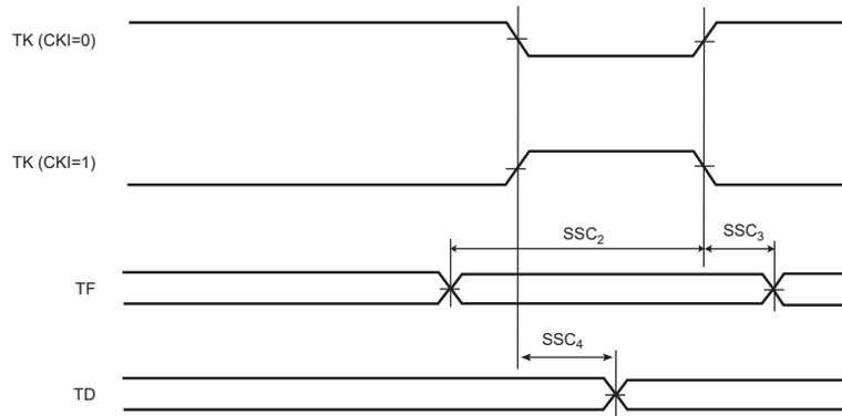
**Figure 59-34. SSC Transmitter, TK and TF in Input**
