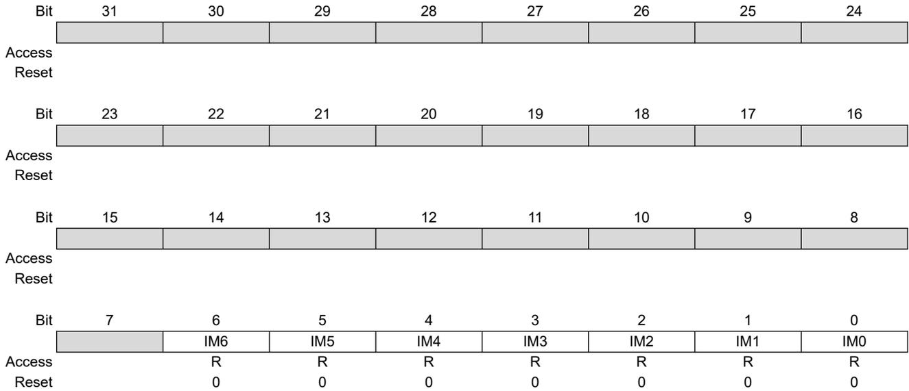
**Bits 0, 1, 2, 3, 4, 5, 6 – IM** XDMAC Channel x Interrupt Mask
