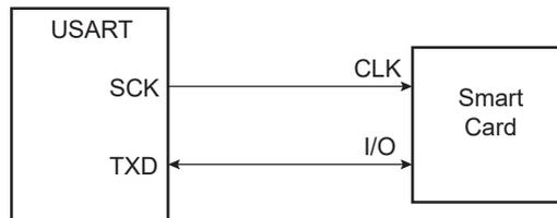
When operating in ISO7816, either in T = 0 or T = 1 modes, the character format is fixed. The configuration is 8 data bits and 1 or 2 stop bits, regardless of the values programmed in the Mode register fields `CHRL`, `MODE9` and `CHMODE`. `US_MR.MSBF` can be used to transmit LSB or MSB first. The bit `INVDATA` can be used to transmit in Normal or Inverse mode. See [46.7.3. US\\_MR](#).
