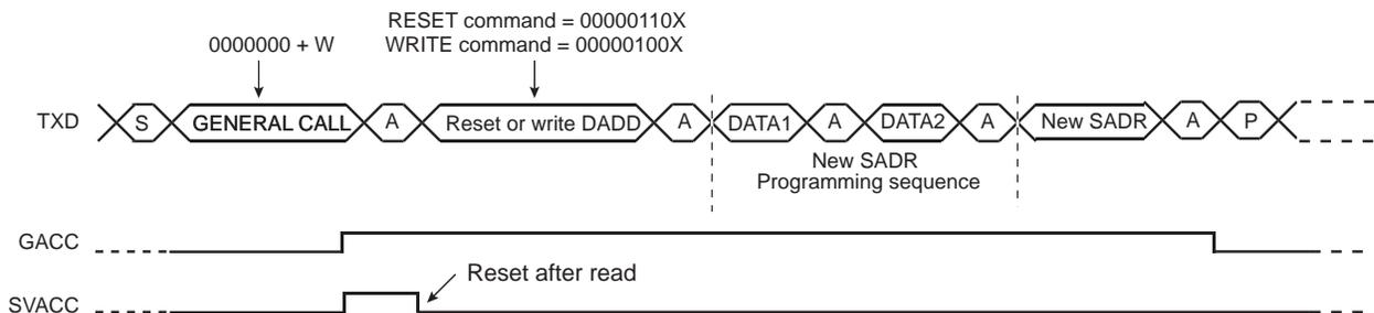
**Note:** This method enables the user to create a personal programming sequence by choosing the programming bytes and their number. The programming sequence has to be provided to the Host.
