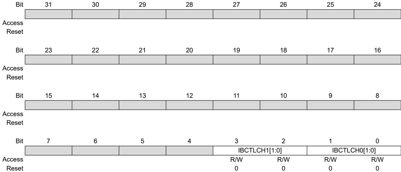
**Bits 0:1, 2:3 – IBCTLCHx** Analog Output Current Control
