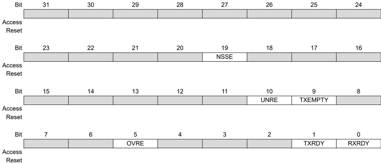
**Bit 19 – NSSE** NSS Line (Driving CTS Pin) Rising or Falling Edge Event Interrupt Enable
