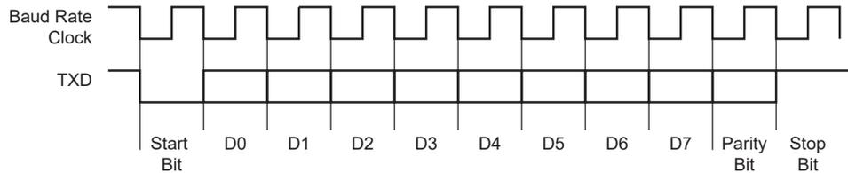
The characters are sent by writing in US\_THR. The transmitter reports two status bits in the Channel Status register (US\_CSR): TXRDY (Transmitter Ready), which indicates that US\_THR is empty, and TXEMPTY, which indicates that all the characters written in US\_THR have been processed. When the current character processing is completed, the last character written in US\_THR is transferred into the Shift register of the transmitter and US\_THR becomes empty, thus TXRDY rises.
