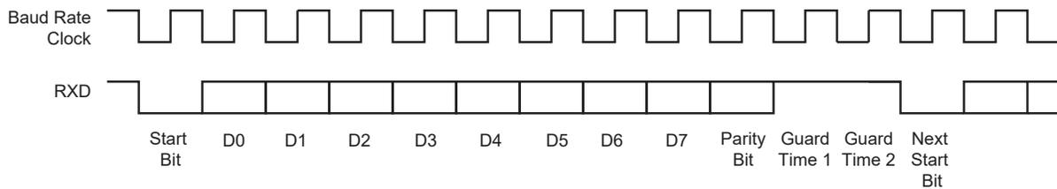
**Figure 46-31. T = 0 Protocol with Parity Error**
