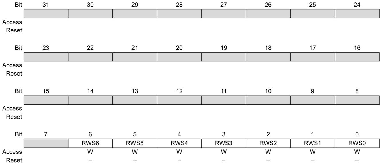
**Bits 0, 1, 2, 3, 4, 5, 6 – RWSx** XDMAC Channel x Read Write Suspend
