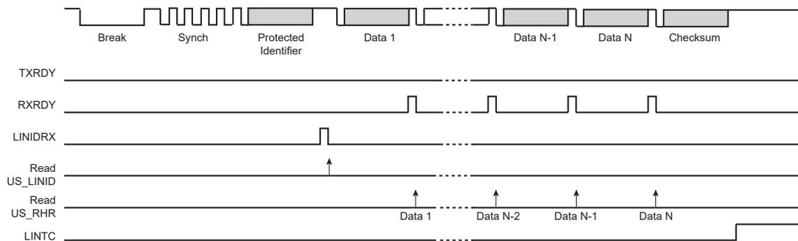
Figure 46-50. Client Node Configuration, NACT = IGNORE
