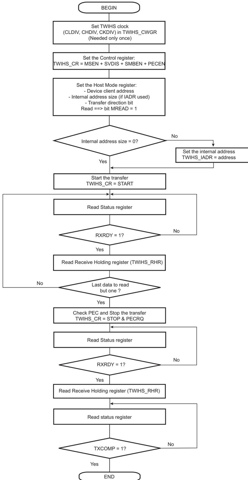
**Figure 43-25. TWIHS Read Operation with Multiple Data Bytes with Alternative Command Mode with PEC**
