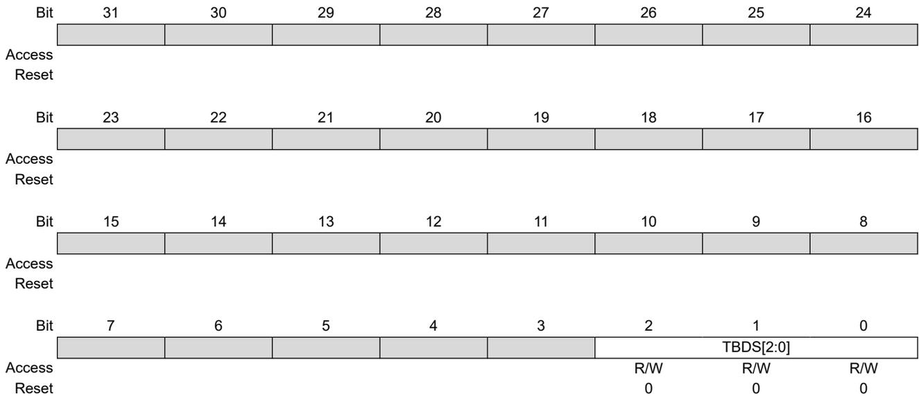
**Bits 2:0 – TBDS[2:0]** Tx Buffer Data Field Size
