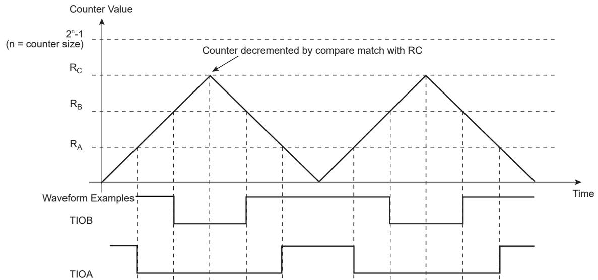
**Figure 50-15. WAVSEL = 11 with Trigger**
