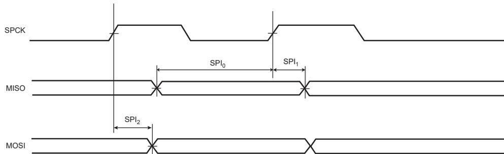
**Figure 59-21. SPI Host Mode with (CPOL = 0 and NCPHA=1) or (CPOL=1 and NCPHA= 0)**
