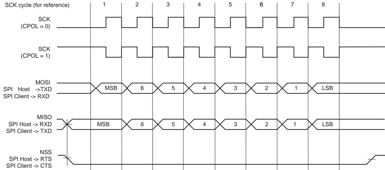
**Figure 46-38. SPI Transfer Format (CPHA = 0, 8 bits per transfer)**
