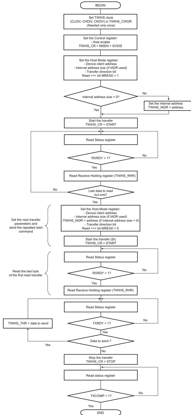
**Figure 43-27. TWIHS Read Operation with Multiple Data Bytes + Write with Alternative Command Mode with PEC**
