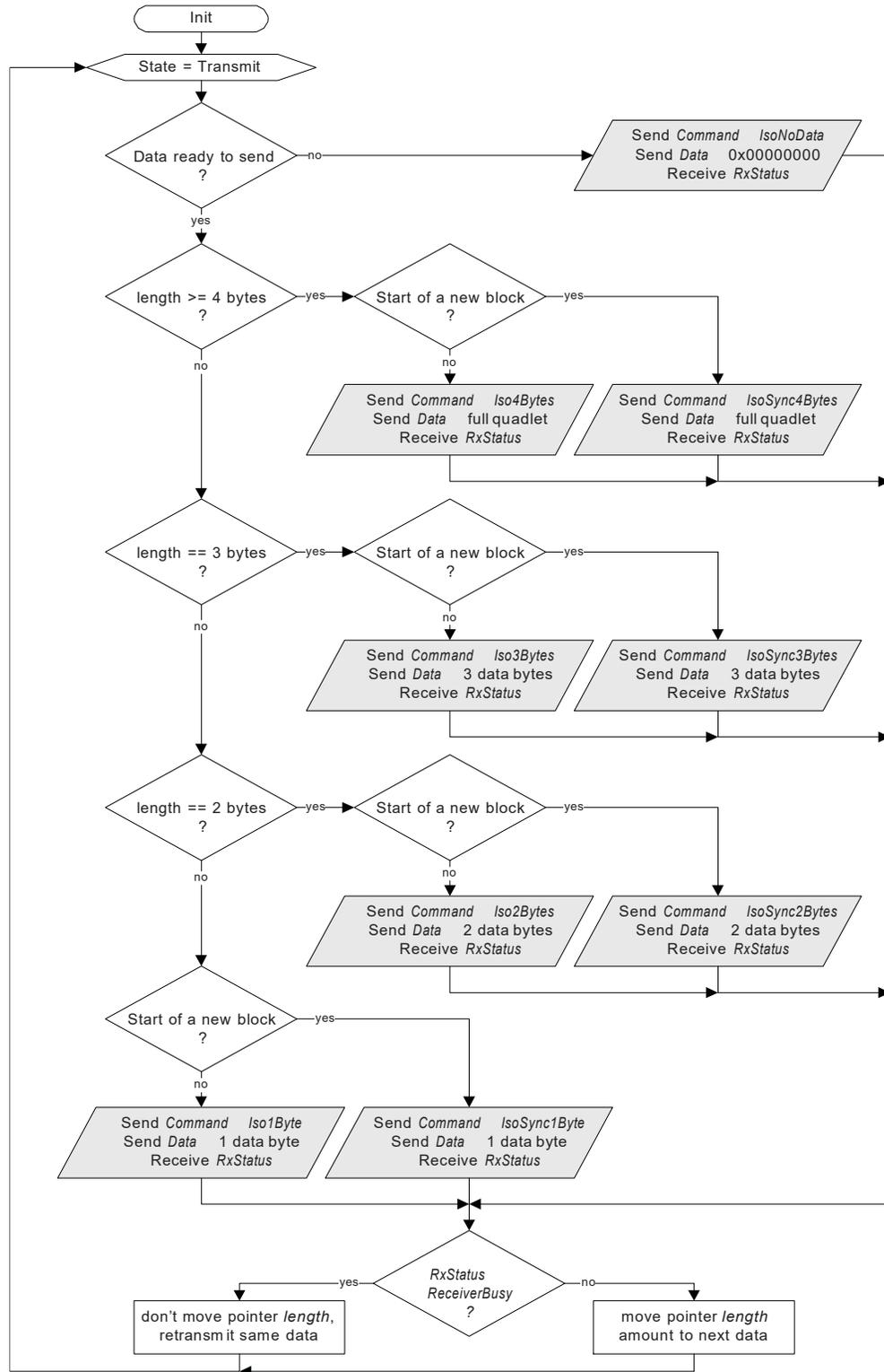
**Figure 48-15. Isochronous Data Rx Device Protocol**
