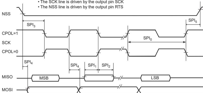
**Figure 58-27. USART SPI Client Mode (Mode 1 or 2)**
