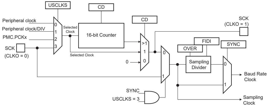
46.6.1.1 Baud Rate in Asynchronous Mode
