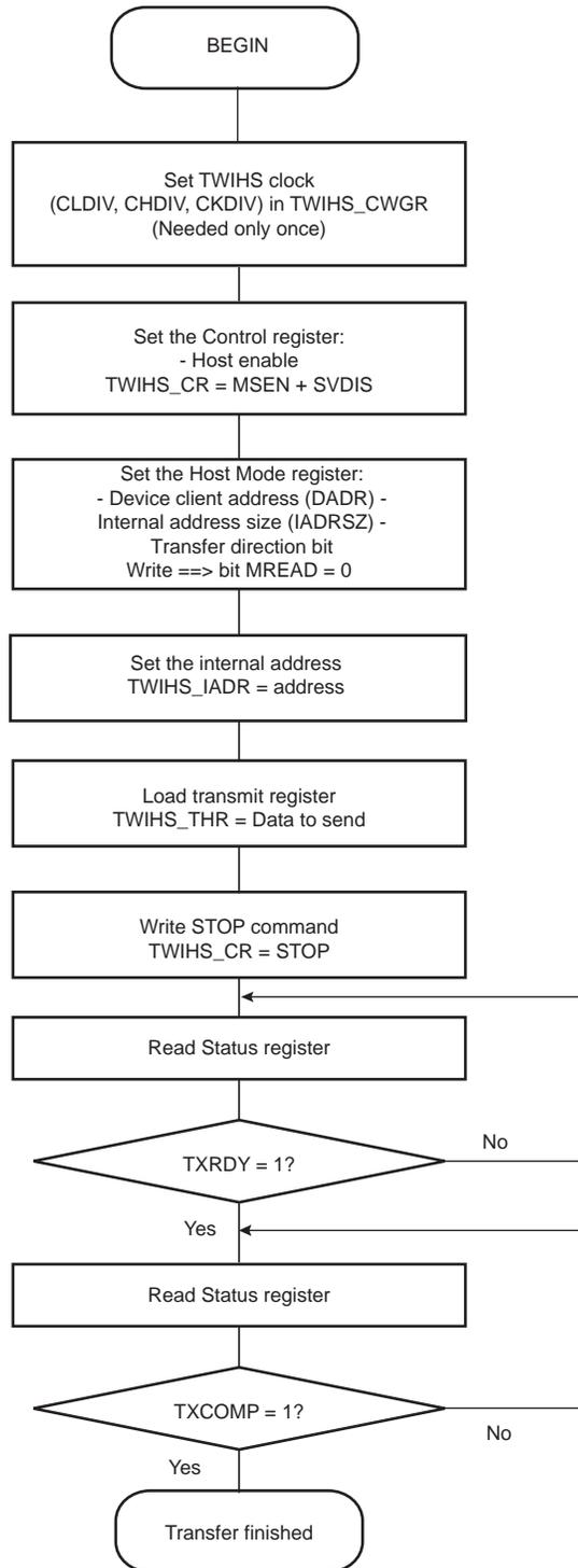
**Figure 43-16. TWIHS Write Operation with Multiple Data Bytes with or without Internal Address**
