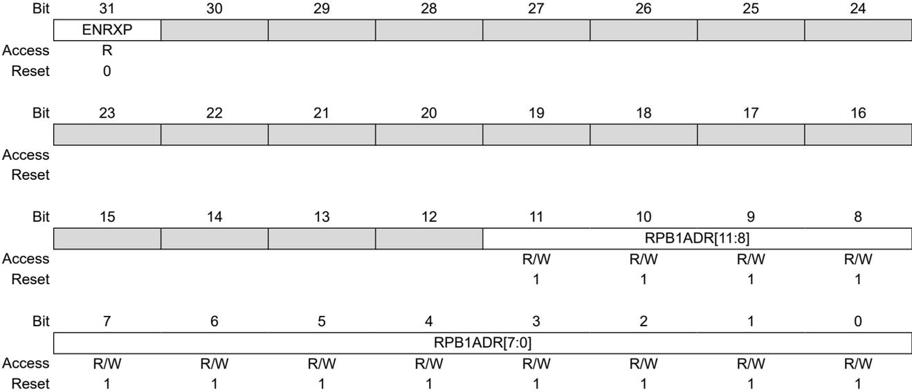
**Bit 31 – ENRXP** Enable RX Partial Store and Forward Operation
