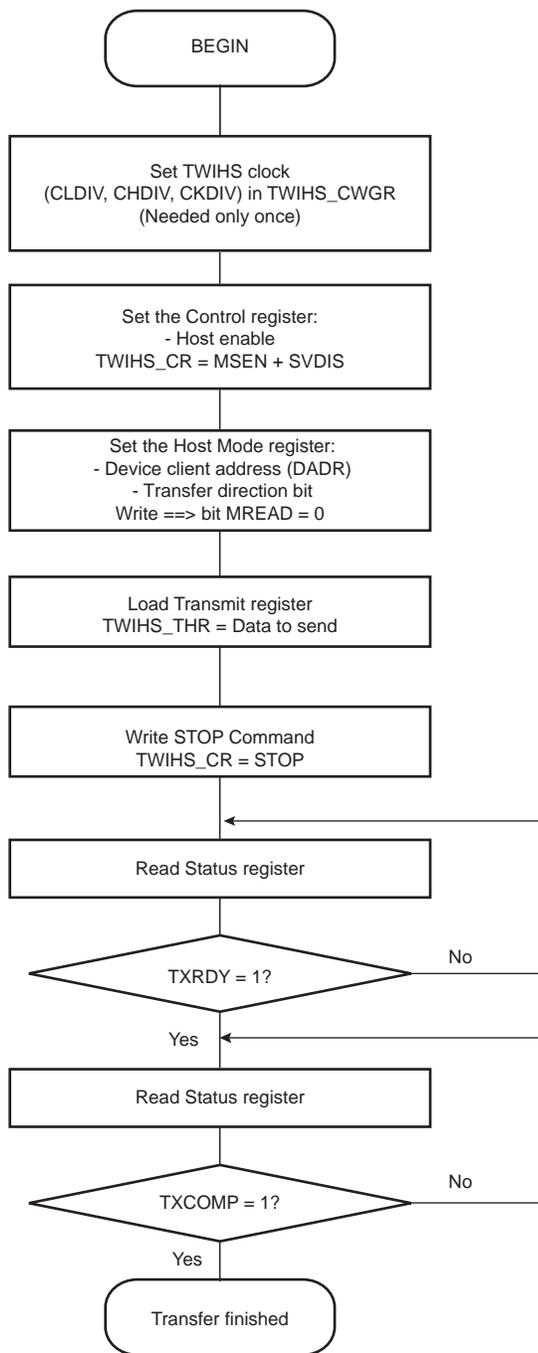
**Figure 43-15. TWIHS Write Operation with Single Data Byte and Internal Address**
