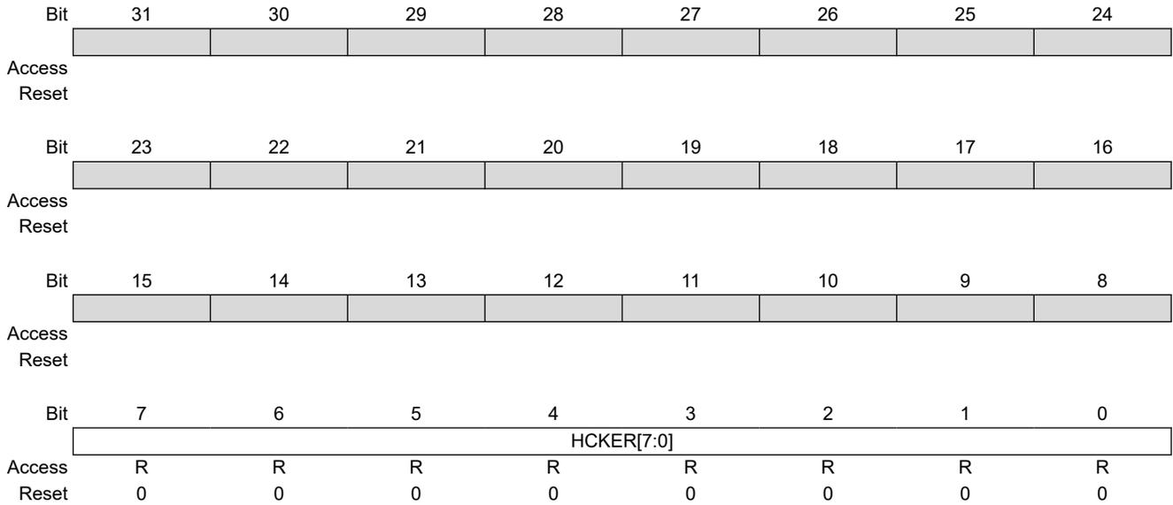
**Bits 7:0 – HCKER[7:0] IP Header Checksum Errors**
