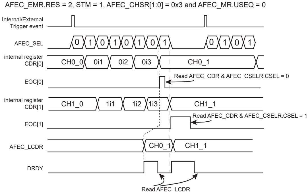
When USEQ is set, the user can define the channel sequence to be converted by configuring AFEC\_SEQxR and AFEC\_CHER so that channels are not interleaved during the averaging period. Under these conditions, a sample is defined for each end of conversion as described in the figure below.
