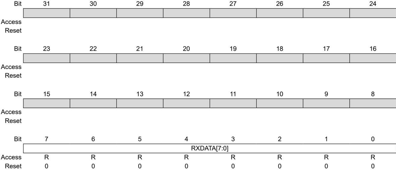
**Bits 7:0 – RXDATA[7:0]** Host or Client Receive Holding Data
