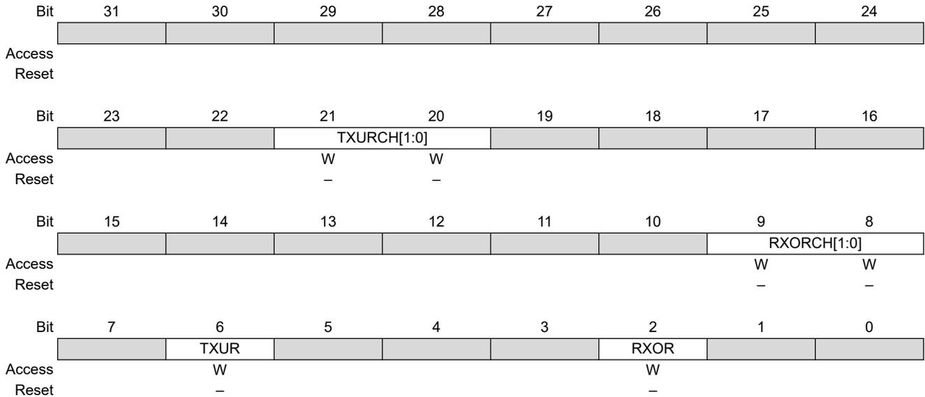
**Bits 21:20 – TXURCH[1:0]** Transmit Underrun Per Channel Status Clear
