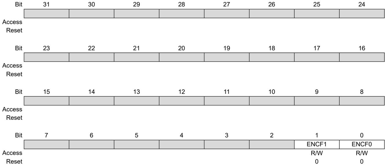
**Bit 1 – ENCF1** Enable Compare Fault Channel 1
