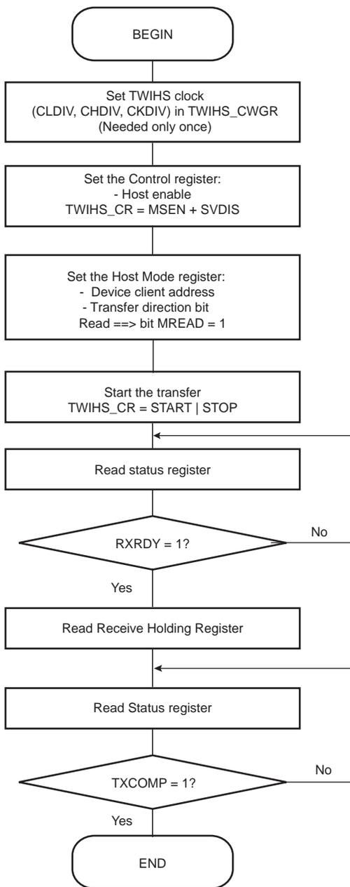
**Figure 43-22. TWIHS Read Operation with Single Data Byte and Internal Address**
