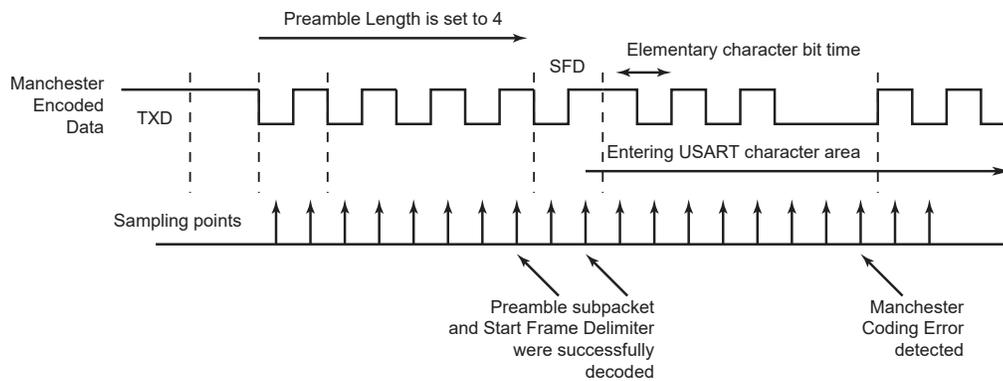
When the start frame delimiter is a sync pattern (US\_MR.ONEBIT = 0), both command and data delimiter are supported. If a valid sync is detected, the received character is written in RXCHR in the Receive Holding register (US\_RHR) and RXSYNH is updated. RXSYNH is set to '1' when the received character is a command, and to '0' if the received character is a data. This alleviates and simplifies the direct memory access as the character contains its own sync field in the same register.
