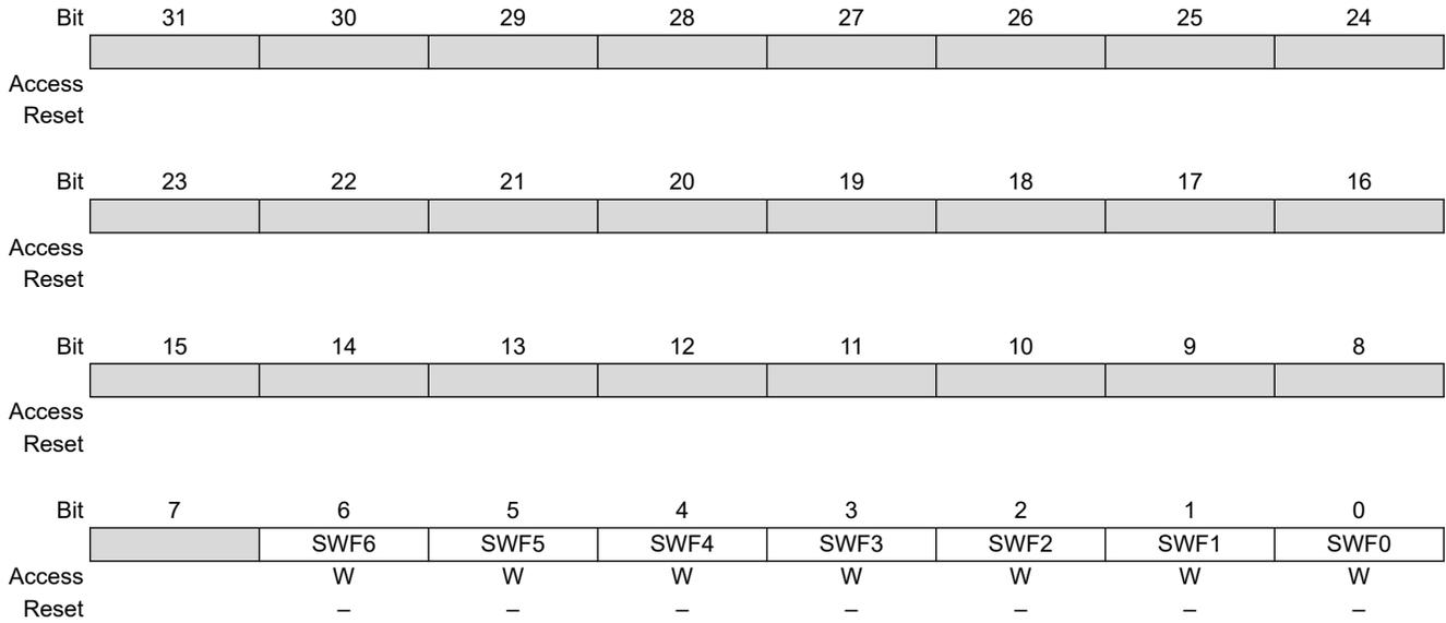
**Bits 0, 1, 2, 3, 4, 5, 6 – SWF<sub>x</sub> XDMAC Channel x Software Flush Request**
