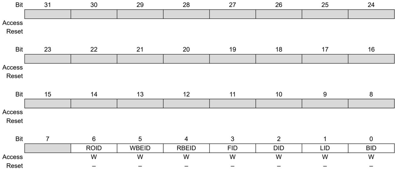
**Bit 6 – ROID** Request Overflow Error Interrupt Disable Bit
