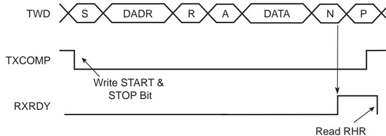
**Figure 43-8. Host Read with Multiple Data Bytes**
