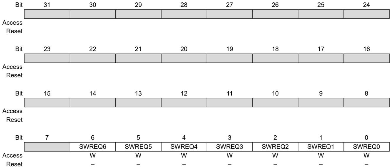
**Bits 0, 1, 2, 3, 4, 5, 6 – SWREQ** XDMAC Channel x Software Request
