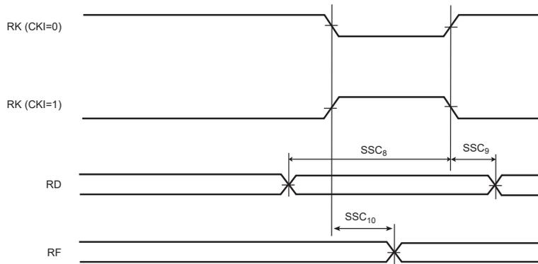
**Figure 58-39. SSC Receiver, RK and RF in Output**
