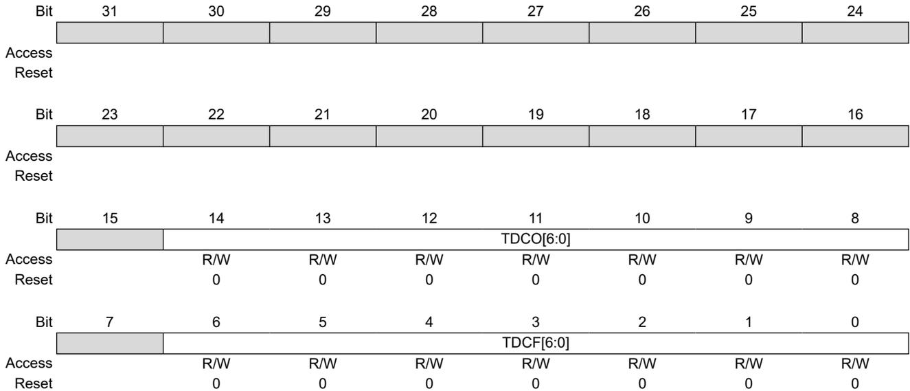
**Bits 14:8 – TDCO[6:0]** Transmitter Delay Compensation Offset
