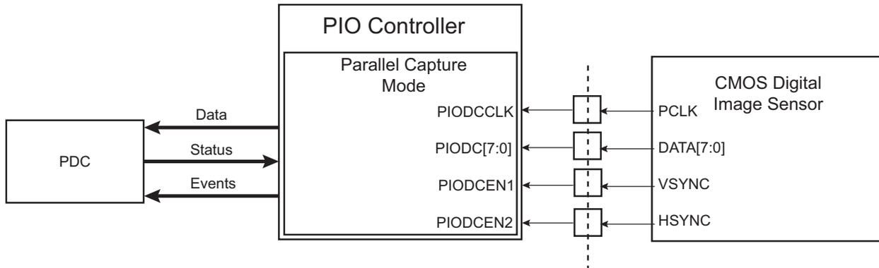
As soon as the Parallel Capture mode is enabled by writing a one to the PCEN bit in PIO\_PCMR, the I/O lines connected to the sensor clock (PIODCCCLK), the sensor data (PIODC[7:0]) and the sensor data enable signals (PIODCEN1 and PIODCEN2) are configured automatically as inputs. To know which I/O lines are associated with the sensor clock, the sensor data and the sensor data enable signals, refer to the I/O multiplexing table(s) in the section “Package and Pinout”.
