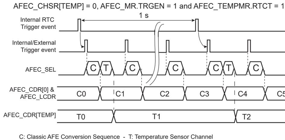
Assuming AFEC\_CHSR[0] = 1 and AFEC\_CHSR[TEMP] = 1 where TEMP is the index of the temperature sensor channel
