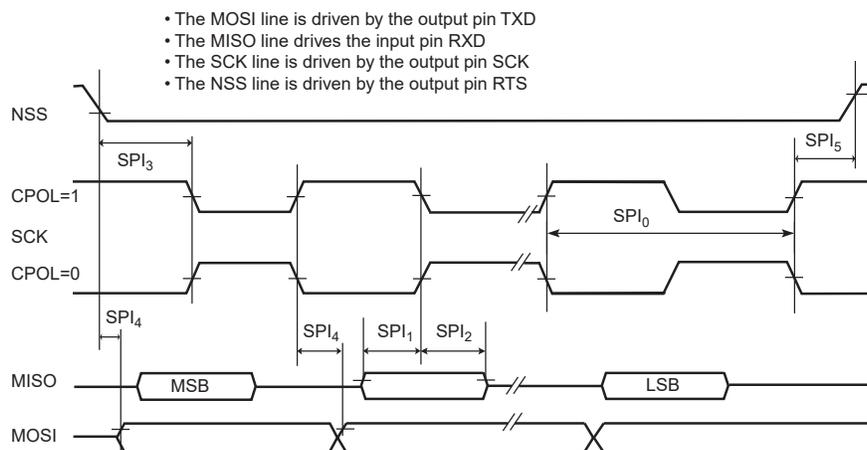
**Figure 59-25. USART SPI Client Mode (Mode 1 or 2)**
