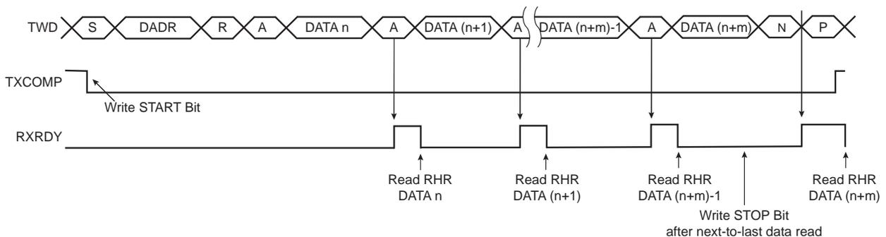
**Figure 43-9. Host Read Clock Stretching with Multiple Data Bytes**
