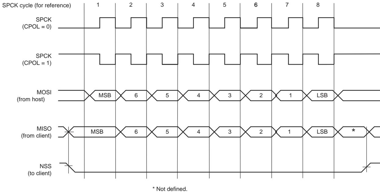
**Figure 41-4. SPI Transfer Format (NCPHA = 0, 8 bits per transfer)**
