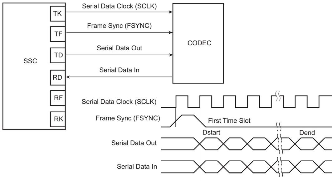
**Figure 44-5. Time Slot Application Block Diagram**
