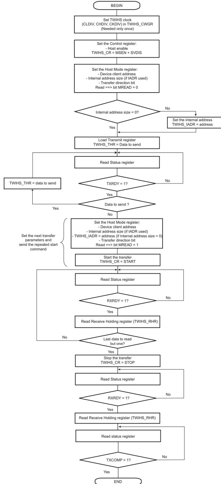
**Figure 43-20. TWIHS Write Operation with Multiple Data Bytes + Read Operation and Alternative Command Mode + PEC**
