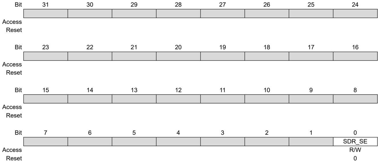
**Bit 0 – SDR\_SE SDRAM Memory Controller Scrambling Enable**
