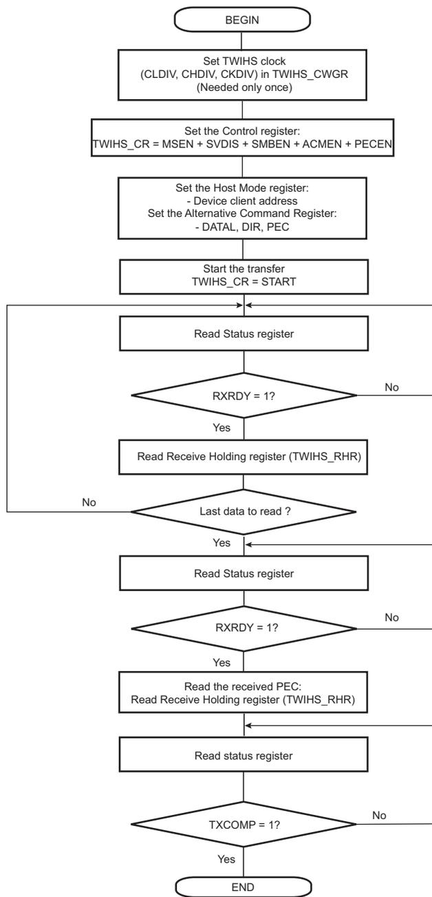
**Figure 43-26. TWIHS Read Operation with Multiple Data Bytes + Write Operation with Multiple Data Bytes (Sr)**
