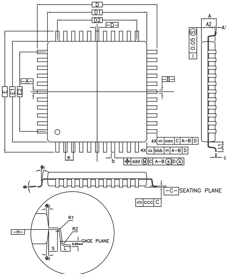
COTROL DIMENSIONS ARE IN MILLIMETERS.
