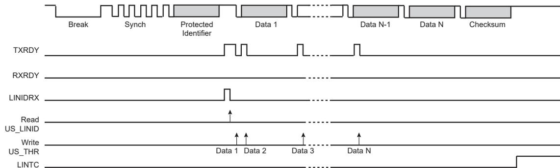
**Figure 46-49. Client Node Configuration, NACT = SUBSCRIBE**
