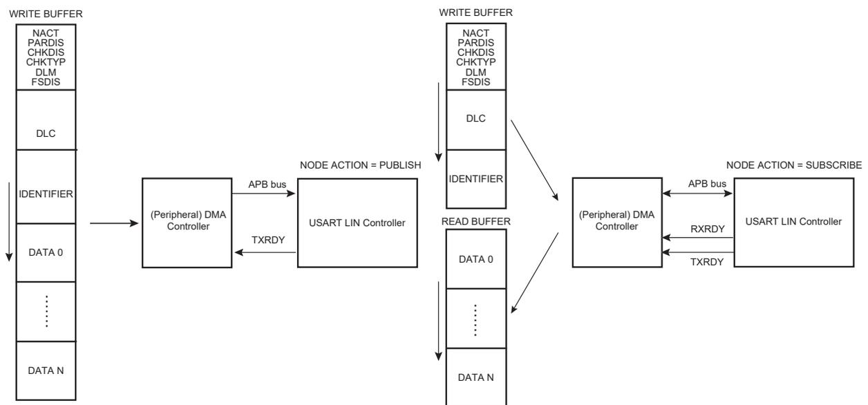
Figure 46-52. Host Node with DMAC (PDCM = 0)
