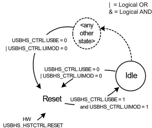
After a hardware reset, the USBHS Device mode is in Reset state. In this state:
