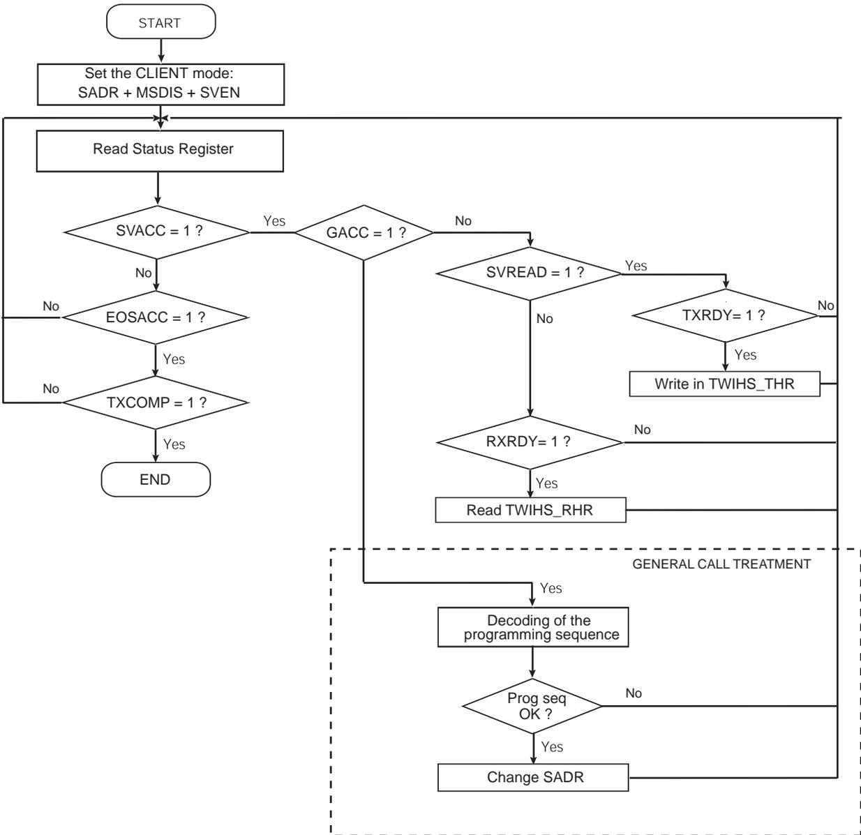
**Figure 43-44. Read Write Flowchart in Client Mode with SMBus PEC**
