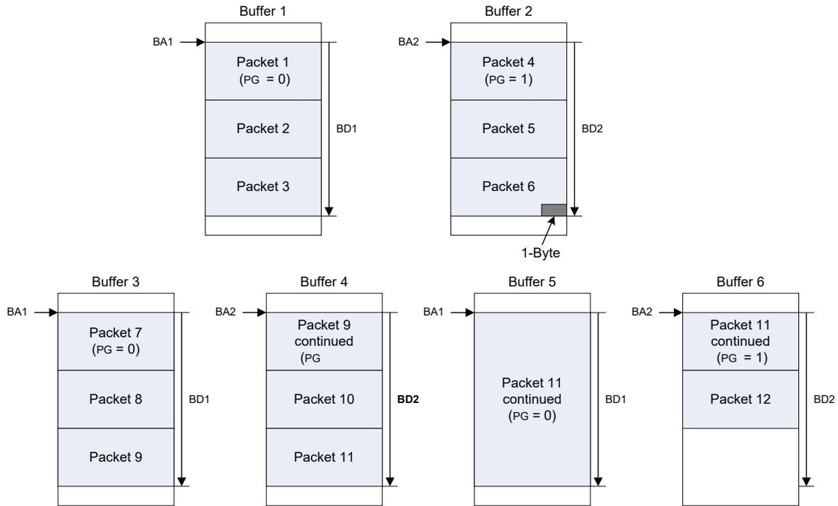
**Table 48-24. Multiple-packet Asynchronous and Control Entry Format**
