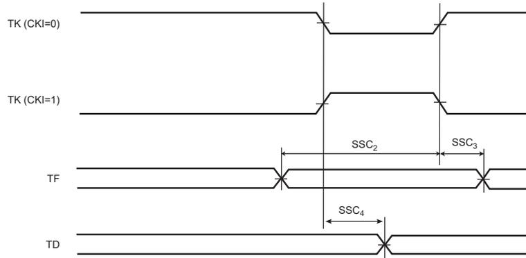
**Figure 58-36. SSC Transmitter, TK and TF in Input**
