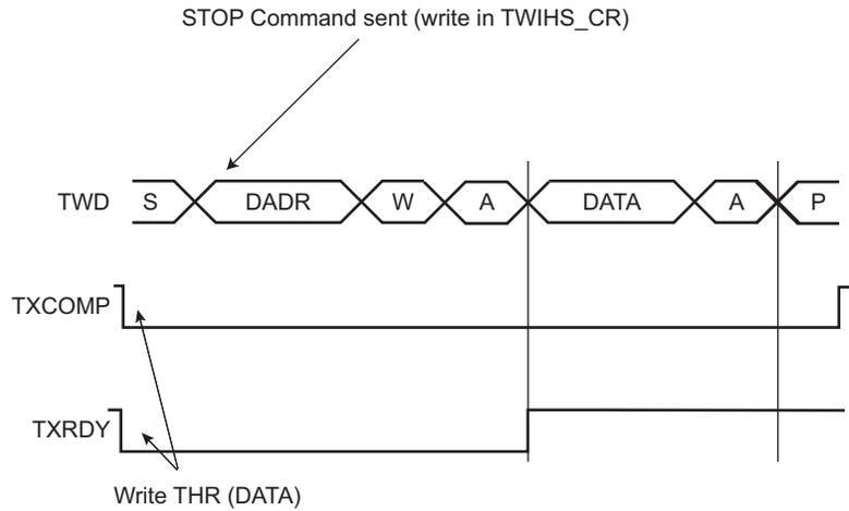
**Figure 43-5. Host Write with Multiple Data Bytes**
