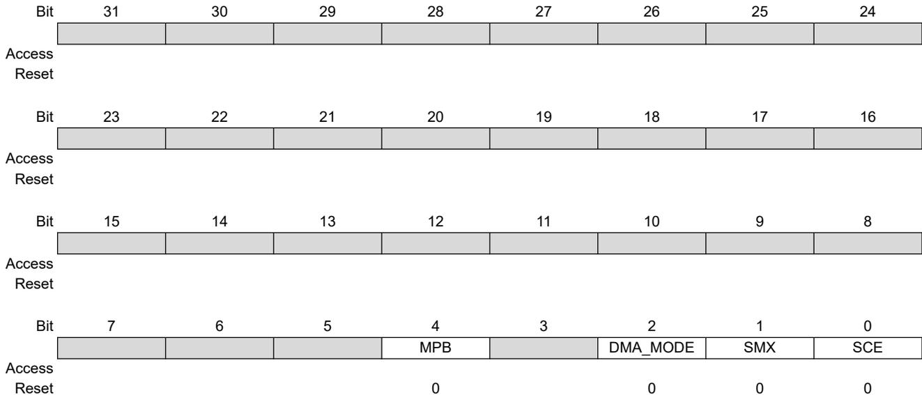
**Bit 4 – MPB** DMA Packet Buffering Mode
