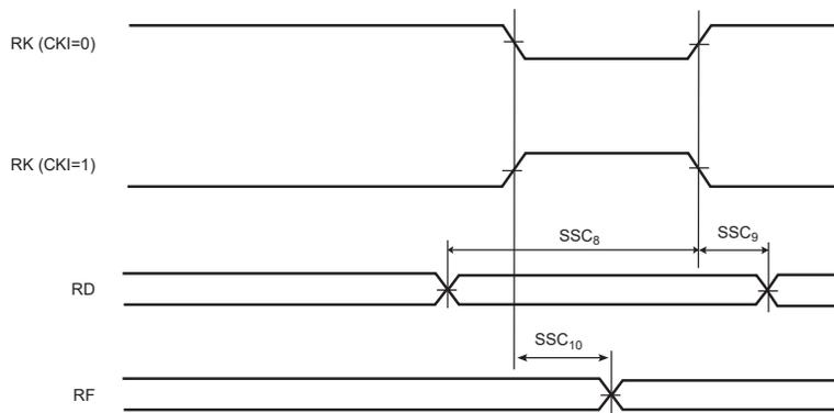
**Figure 59-37. SSC Receiver, RK and RF in Output**
