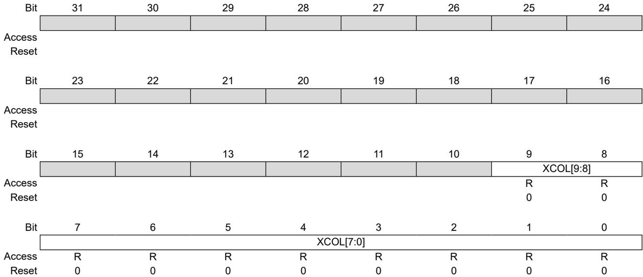
**Bits 9:0 – XCOL[9:0] Excessive Collisions**
