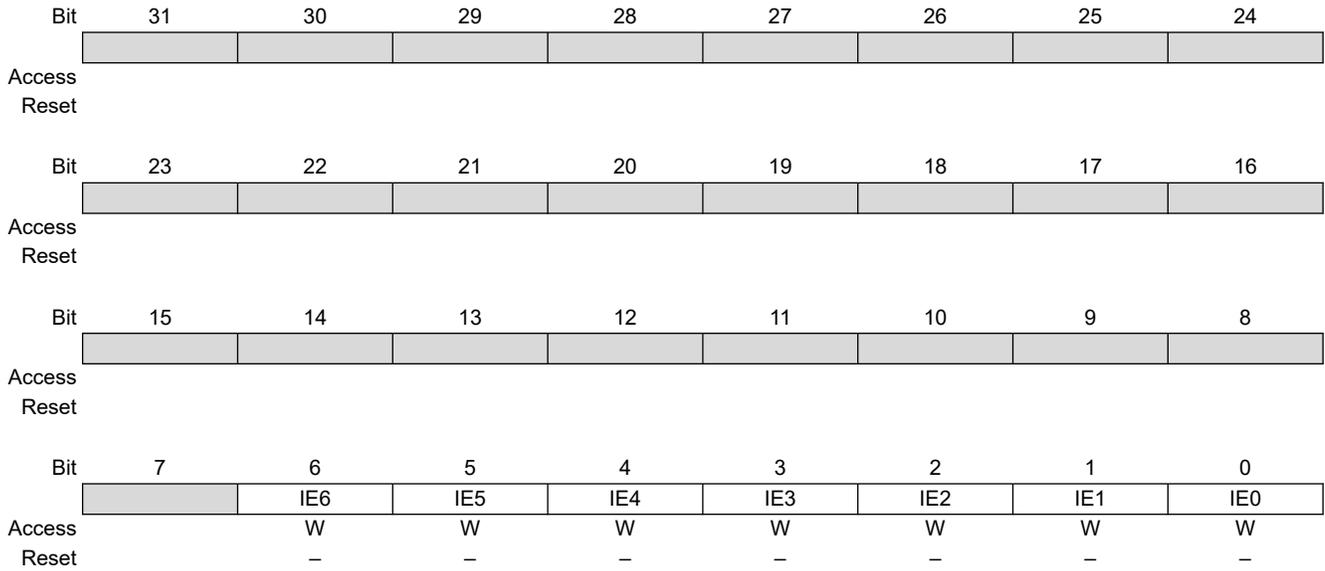
**Bits 0, 1, 2, 3, 4, 5, 6 – IE XDMAC Channel x Interrupt Enable**
