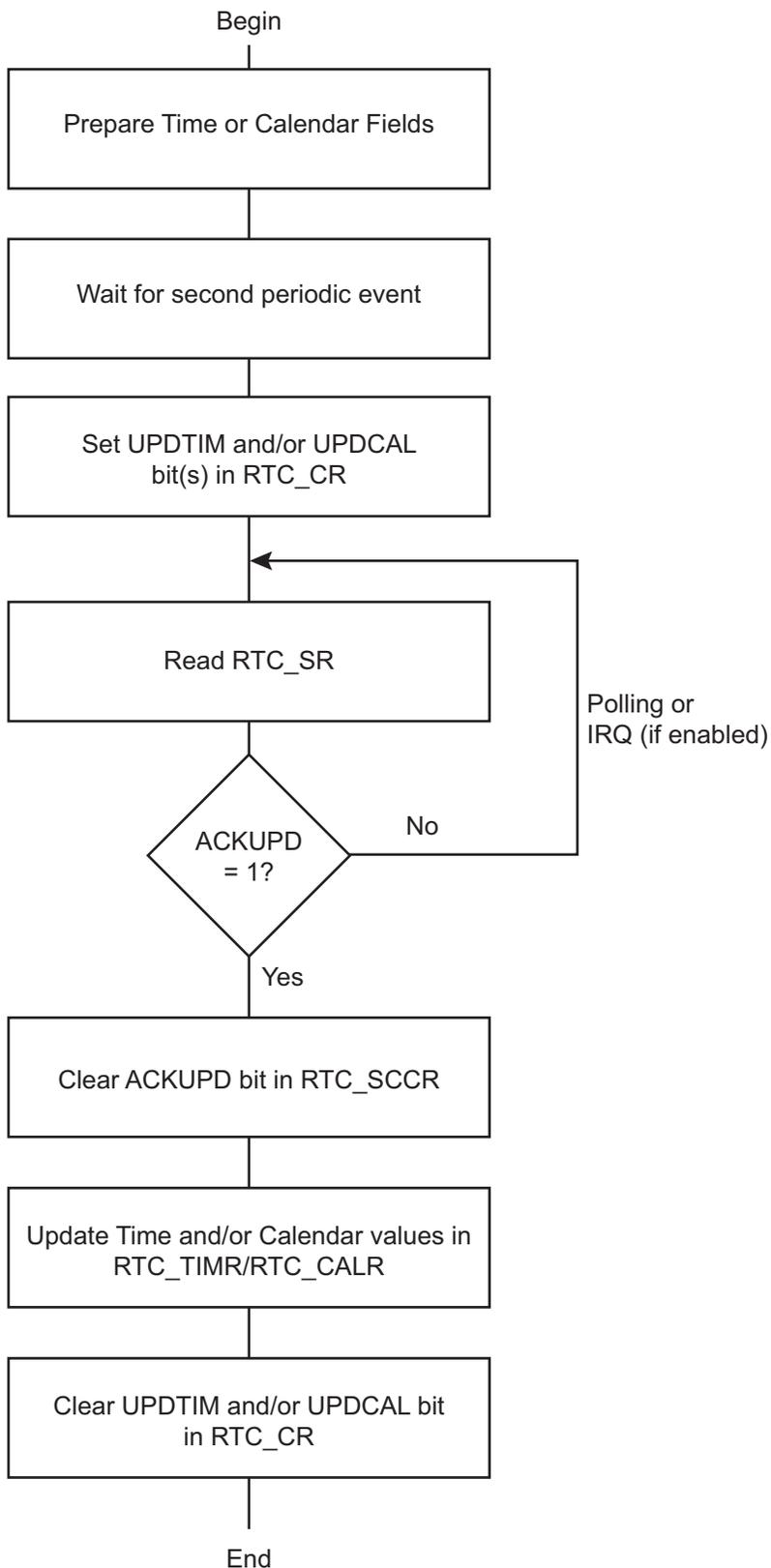
**27.5.7 RTC Accurate Clock Calibration**
