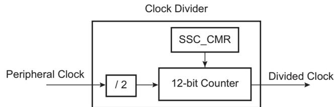
The peripheral clock divider is determined by the 12-bit field DIV counter and comparator (so its maximal value is 4095) in the Clock Mode Register (SSC\_CMR), allowing a peripheral clock division by up to 8190. The Divided Clock is provided to both the receiver and the transmitter. When this field is programmed to 0, the Clock Divider is not used and remains inactive.
