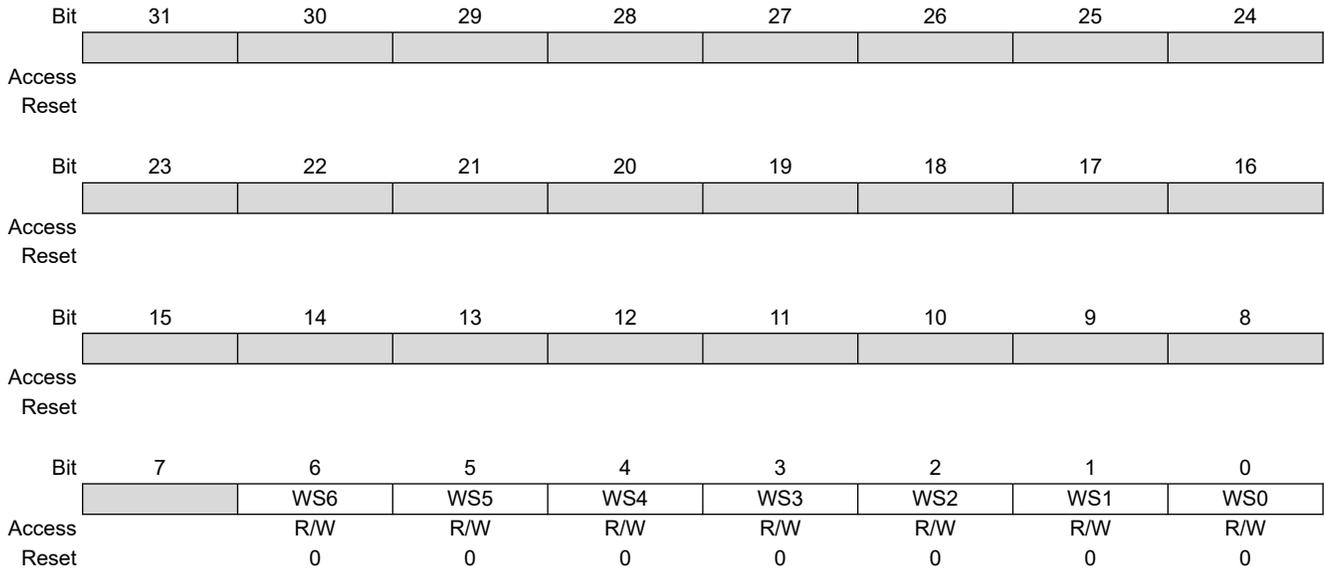
**Bits 0, 1, 2, 3, 4, 5, 6 – WSx XDMAC Channel x Write Suspend**
