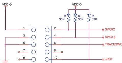
**Figure 60-2. SWD Schematic Example with a 20-pin Connector**
