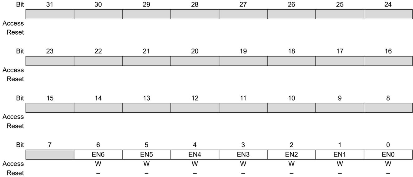
**Bits 0, 1, 2, 3, 4, 5, 6 – EN XDMAC Channel x Enable**
