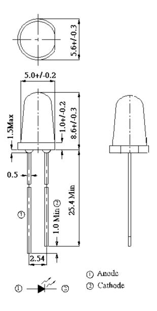
**Notes**: 1.All dimensions are in millimeters 2.Tolerances unless dimensions ±0.25mm
