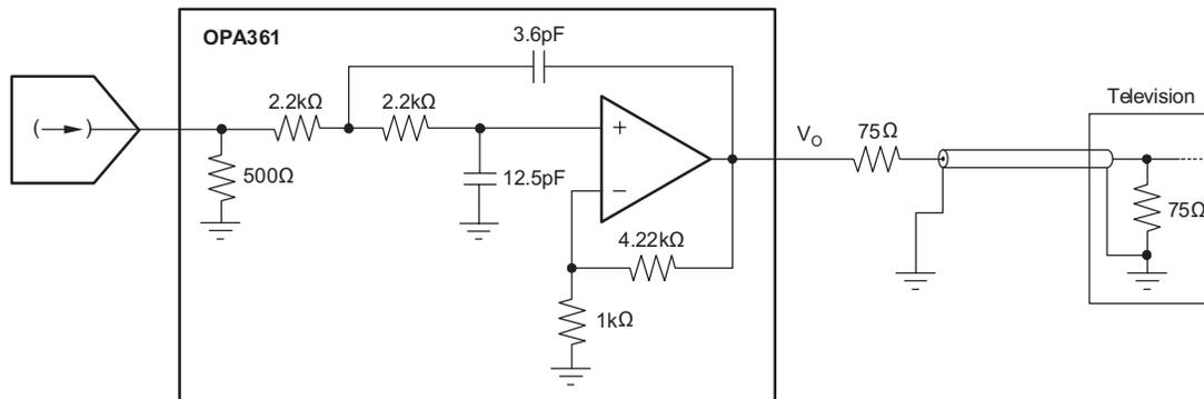
**Figure 2. Filter Structure of the OPA361-Q1**
