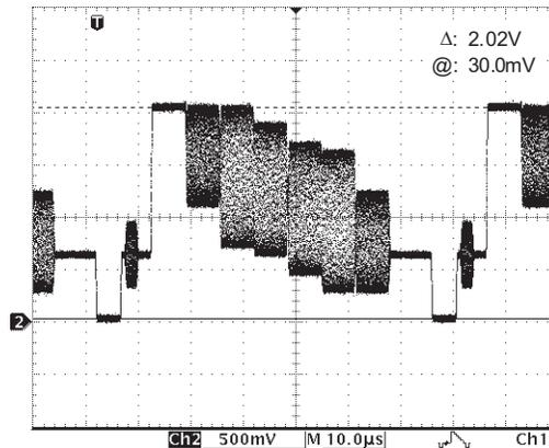
**Figure 3. 100/75 Color Bar Signal at Output of OPA361-Q1**
