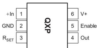
The location of pin 1 on the OPA361-Q1 is determined by orienting the package marking as shown in the diagram above.
