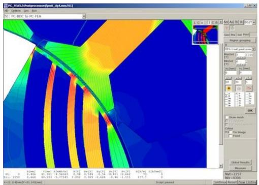
Detail of a synchronous reluctance motor showing the multi-layer structure and the saturable bridges in the rotor. *Image courtesy of CD-adapco*.
