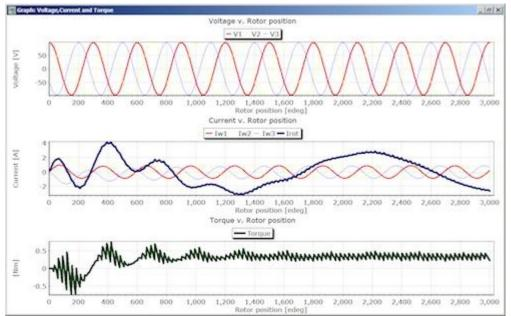
This SPEED image depicts the transient calculation for an induction machine in which the inductances of the stator coils and rotor bars are calculated individually instead of using the classical equivalent circuit. This new method is said to avoid the simplifying assumptions made in the classical theory in relation to the effect of space harmonic effects. *Image courtesy of CD-adapco*.
