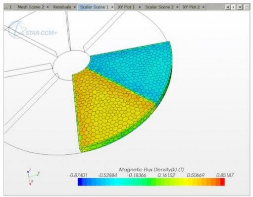
SPEED version 2011 can now transfer many geometries to STAR-CCM+ directly. This color map of flux-densities in STAR-CCM+ shows two magnets in an axial-flux motor. *Image courtesy of CD-adapco*.
