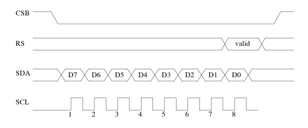
2.5.2 Access to Display RAM and Internal Register
