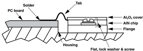
The area under the device should be flat to less than 0.001" and free of burrs and scratches. For maximum heat transfer from the device to the heat sink use either thermal grease or a thermal gasket. Keep the thickness of the grease to less than 0.002". Be sure to form a small loop in the tab, making sure you support it while doing so. This will act as a strain relief as the heat
