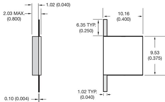
**Mechanical Tolerance:** ±0.25 (0.010) unless otherwise specified
