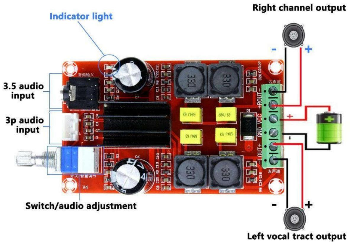
**Warm hint: the red line is the positive pole, the black line is negative, do not connect the reverse power and negative pole, please do not use the power and power size of the sound.**
