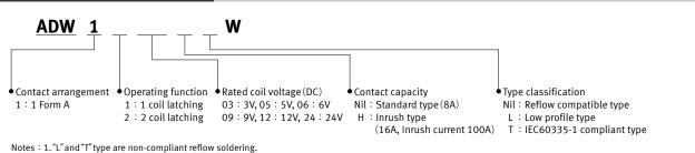
Notes : 1. "L" and "T" type are non-compliant reflow soldering 2.1 ow profile type is available (inrush type only).
