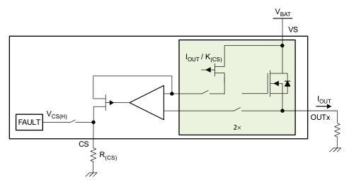
Figure 24. Current-Sense Block Diagram
