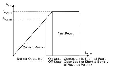
Figure 25. Current-Sense Output-Voltage Curve
