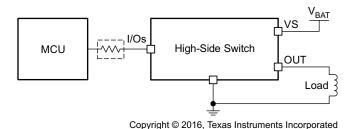
Figure 35. MCU I/O External Protection
