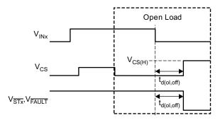
Figure 3. Open-Load Blanking-Time Characteristics
