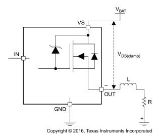
Figure 27. Drain-to-Source Clamping Structure
