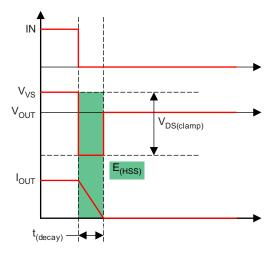
Figure 28. Inductive Load Switching-Off Diagram
