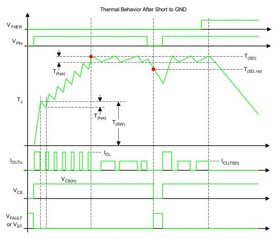
Figure 31. Thermal Behavior Diagram
