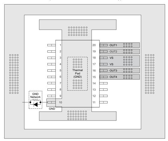
Figure 44. Layout Example With a GND Network
