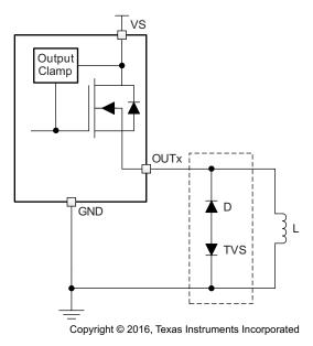
Figure 29. Protection With External Circuitry
