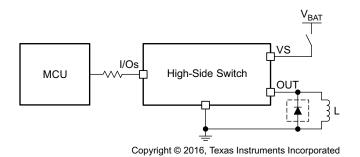
Figure 32. Protection for Loss of Power Supply
