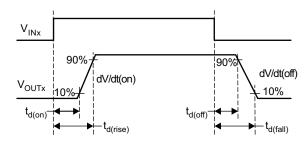
Figure 1. Output Delay Characteristics
