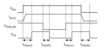
Figure 2. CS Delay Characteristics
