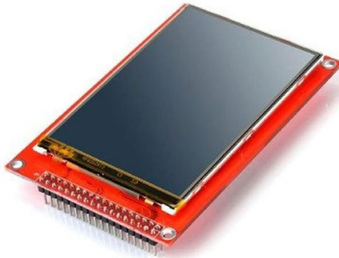
This TFT display is big (3.5" diagonal) bright and colorful! 480×320 pixels with individual RGB pixel control, this has way more resolution than a black and white 128×64 display, and double our 2.8" TFT.
