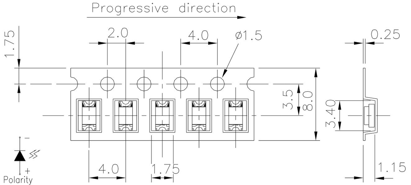
**Note:** Tolerances Unless Dimension is  $\pm 0.1\text{mm}$ , Unit = mm
