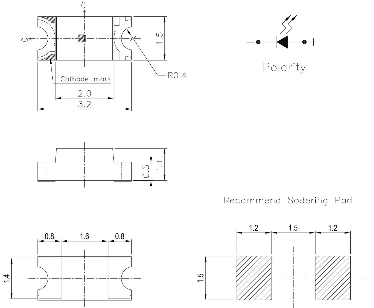
**Note:** Tolerances Unless Dimension is  $\pm 0.1\text{mm}$ , Unit = mm
