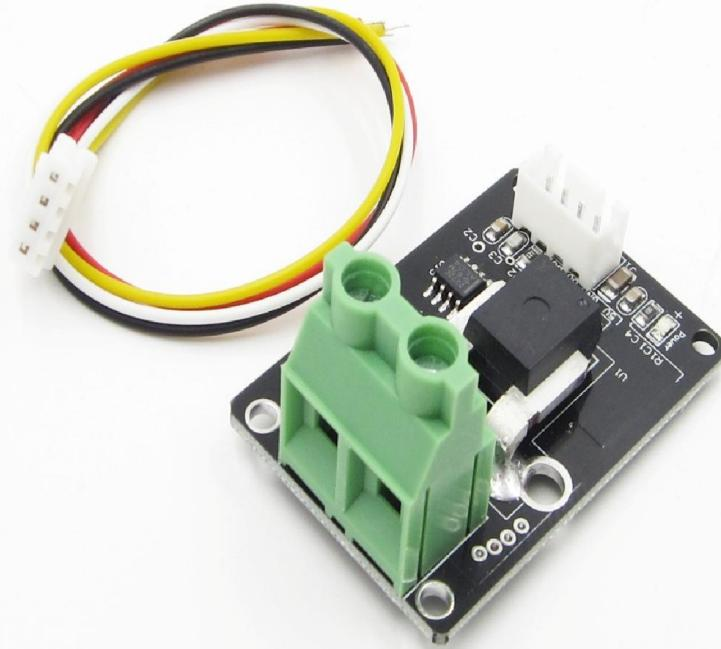
**Bidirectional Current Sens module 120 kHz Bandwidth DC: -100-100A 0.02V/1A
