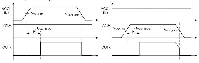
Figure 31. VCCI Power-up UVLO Delay
