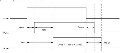
Figure 27. Overlapping Inputs, Dead Time Disabled
