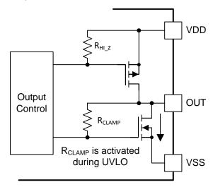
Figure 34. Simplified Representation of Active Pull Down Feature
