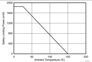
Figure 3. Thermal Derating Curve for Safety-Related Limiting Power
