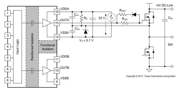
Figure 39. Negative Bias with Zener Diode on Iso-Bias Power Supply Output
