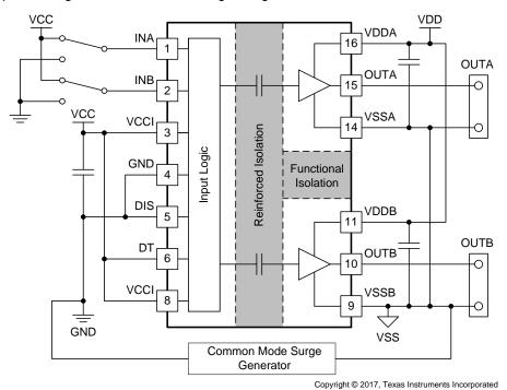
Figure 33. Simplified CMTI Testing Setup
