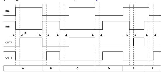
Figure 37. Input and Output Logic Relationship With Input Signals
