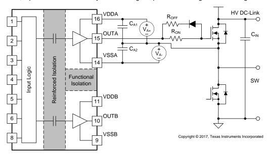
Figure 40. Negative Bias with Two Iso-Bias Power Supplies
