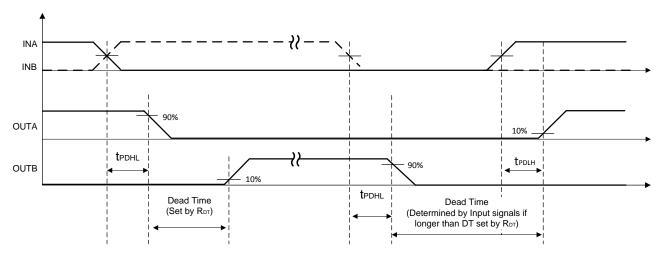
Figure 30. Dead-Time Switching Parameters
