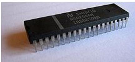
The National Semiconductor [8250 UART](#) chip, one of the most prolific and most cloned [UART chips](#) due to its presence in the first [IBM Personal Computer](#).
