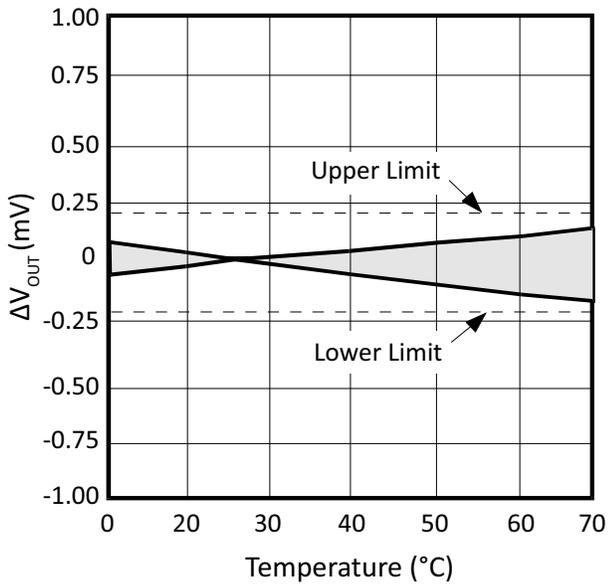
Figure 3:  $V_{OUT}$  vs. Temperature (VRE305C)
