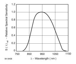
Figure 6. Relative Spectral Sensitivity vs. Wavelength
