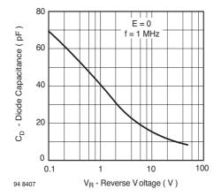
Figure 5. Diode Capacitance vs. Reverse Voltage
