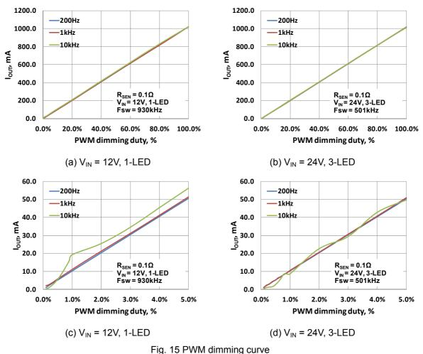
Users can also apply DC voltage directly to DIM for modulating LED current. The result is shown in the following figures.
