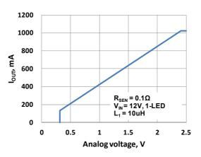
Fig. 16 Analog dimming curve
