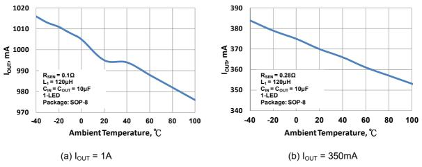
Fig. 12 Output Current vs. Ambient Temperature at  $V_{IN}$  = 12V
