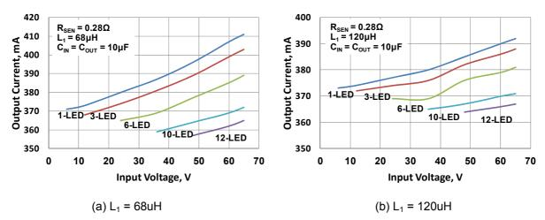
Fig. 8 Output current vs. input voltage at I<sub>OUT</sub> = 350mA
