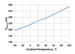
Fig. 13  $R_{ds(on)}$  vs. Ambient Temperature at V<sub>IN</sub> = 12V
