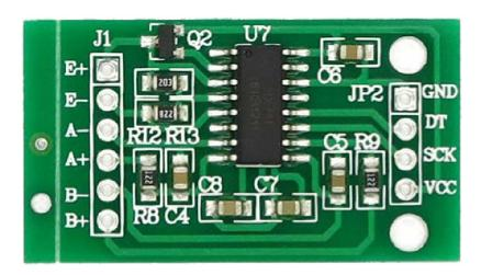
Simply connect Load cell wires to the HX711 module based on their color, then connect DAT (Data) pin to Arduino Analog pin A1 and connect CLK (Clock) pin to Arduino Analog pin A0, Put Vcc and Gnd supply from Arduino power source pins.
