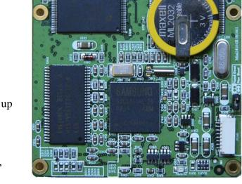
GPIO, Local bus and all I/O CPU lines can be extended via two 4mm height 0.6mm space 140-pin board-to-board connectors.
