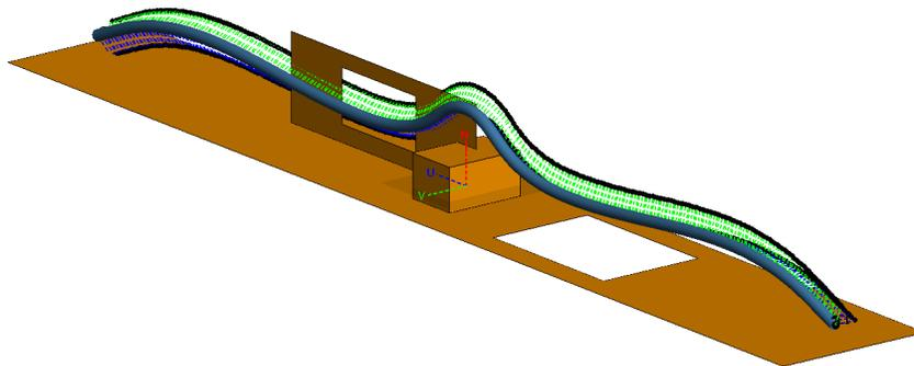
*Figure 10: A preview of the cable cross-section orientation of a cable running above an arbitrary ground installation.*
