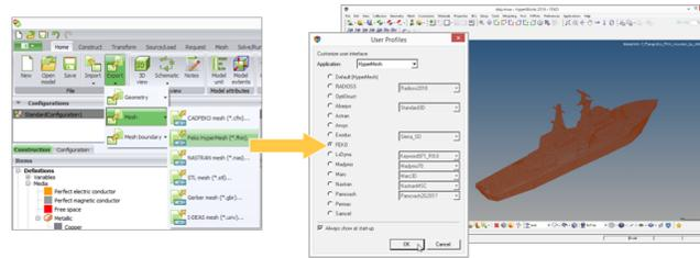
Figure 3: The Feko User Profile in HyperMesh ensures the generation of a valid mesh for Feko.
