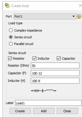
Figure 7: The **Create load** dialog now shows an image of the resulting circuit.
