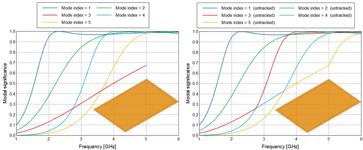
Figure 19: Modal significance plots from a characteristic mode analysis performed on a PEC plate showing tracked modes on the left and untracked results on the right.
