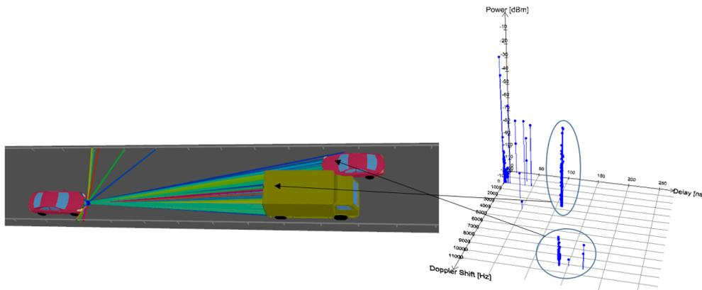
Figure 9: An automotive radar simulation in Altair WinProp.
