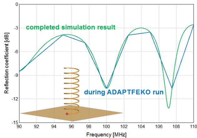
Figure 18: A Cartesian graph with the reflection coefficient of a helix antenna shows the completed continuous frequency result and the discrete result as it gets displayed during simulation.
