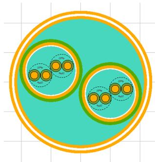
Figure 6: CADFEKO cross-sectional view of a cable bundle with double shields.
