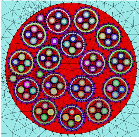
Figure 17: An example of a cable cross section mesh used by the solver.
