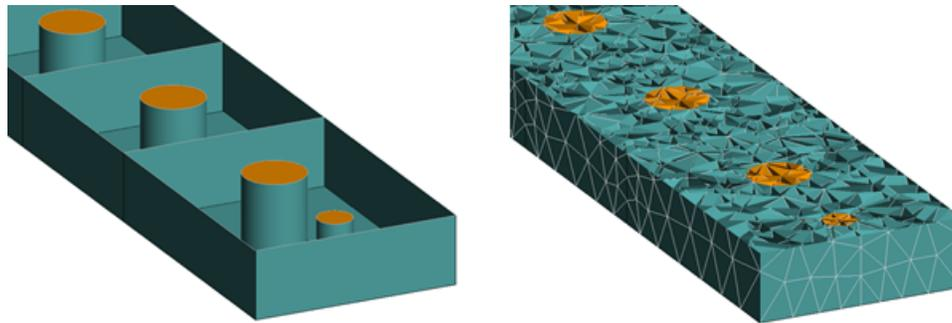
*Figure 20: Partial view of a coaxial diplexer model (left) and mesh (right) with the perfect electric conductor pins meshed into tetrahedra with the dielectrics and solved as part of the FEM solution.*
