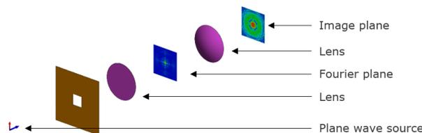
*Figure 1: The optical 4F correlator (dielectric lenses) in the image simulates 16 times faster in Feko 2019 than in Feko 2018.2.1 on a laptop with Nvidia Quadro M1000M GPU.*
