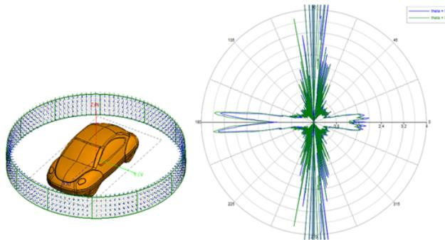
Figure 4: Feko-calculated RCS information can be included in a WinProp simulation through .ffe file import.
