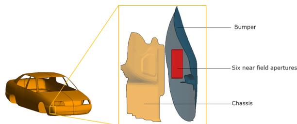
*Figure 2: Side view of a radar antenna placement using 6 near field apertures, located in between the bumper and chassis.*
