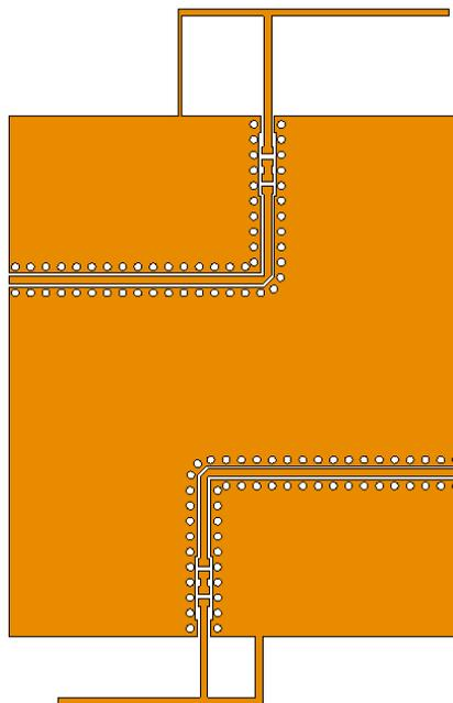
Figure 12: View of an exported Gerber file of a planar antenna with via holes.
