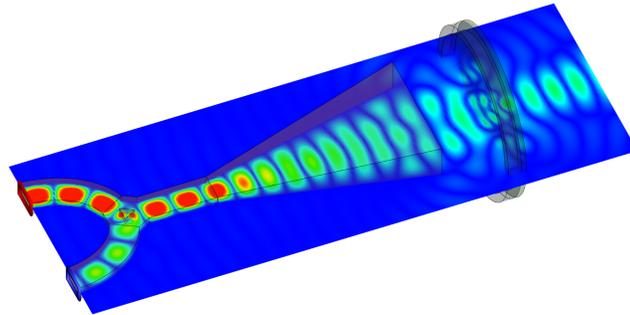
Figure 15: Ferrite circulator (FEM) with horn antenna and dielectric lens (SEP).
