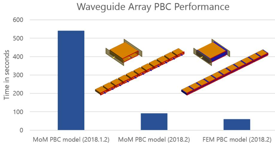
Figure 5: An 11x1 waveguide array solved at 1.645 GHz. The image shows the performance of the MoM PBC array solved with Altair Feko 2018.1.2 compared to the MoM PBC array solved with Altair Feko 2018.2 and the FEM PBC array solved with Altair Feko 2018.2. The PBC unit cells for the MoM and FEM models are shown as inserts with the 3D views of the models. The simulations were completed on a standard desktop computer (Intel® Core™ i5-4690 CPU @ 3.50GHz).
