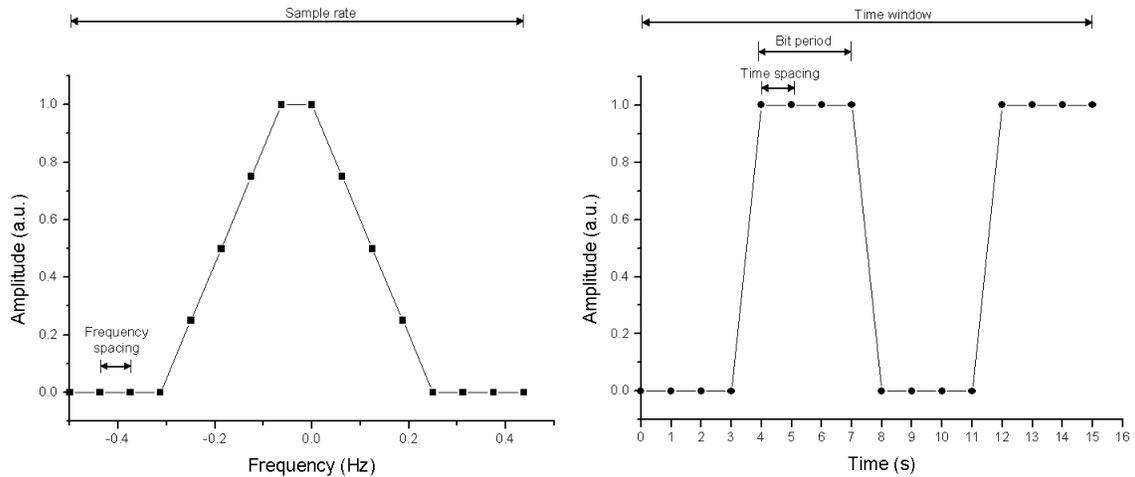
Time spacing =  $1 / \text{Sample rate} = \text{Time window} / \text{Number of samples}$
