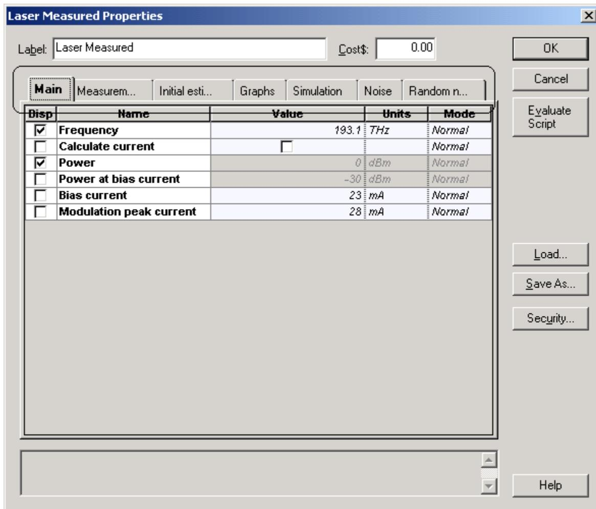
Component parameters are organized by categories. **Laser Measured** has seven parameter categories, each represented by a tab in the dialog box (see [Figure 11](#)).
