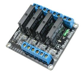
1, OMRON 5V 240V solid state relay 2A, output with resistance type fuse 240V 2A.
