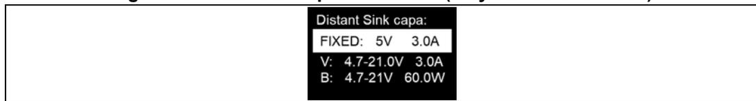
This screen displays the sink profiles. This information is retrieved only in standalone sink mode, because a dedicated command (get sink capabilities) is sent by the G0 disco application. No actions or selection may be triggered here on a distant sink profile.
