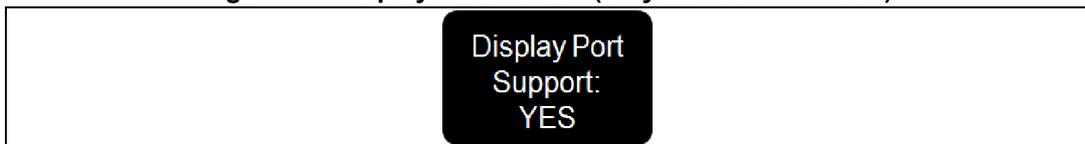
If the source is capable of using the super speed lines to send display port video signal, the information is displayed. This screen also displays if Thunderbolt capability is available. This information is gathered only in standalone sink mode, because the G0 issues a Discovery identity message. In some case, the source may not respond to this message, and therefore no information may be retrieved.
