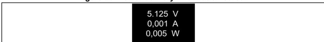
This screen displays the current VBUS power: voltage and current, and calculated power.
