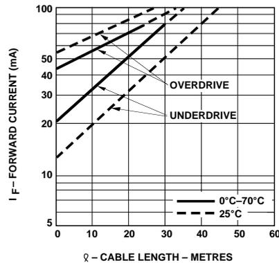
Figure 4. Guaranteed system performance with improved cable (HFBR-15X1/25X1).
