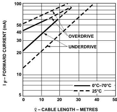
Figure 3. Guaranteed system performance with standard cable (HFBR-15X1/25X1).
