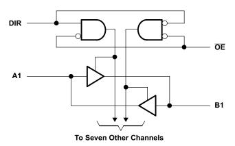
Figure 4. Logic Diagram (Positive Logic)
