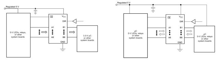
Figure 5. Typical Application Schematic
