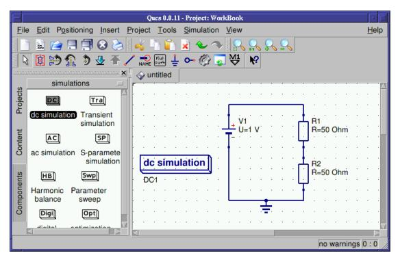
Figure 8: Ground symbol as well as DC simulation in place
