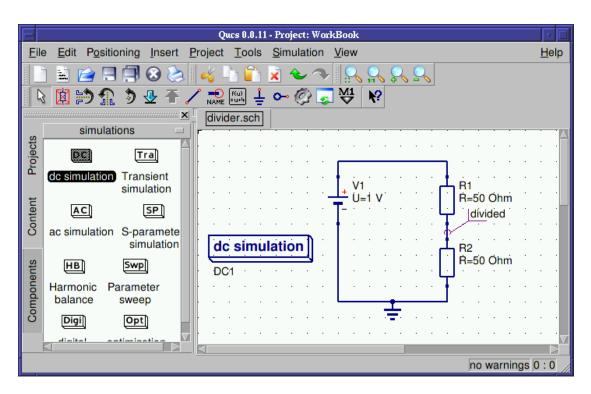
Figure 11: Final voltage divider schematic
