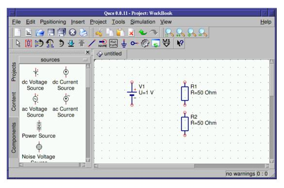
Figure 6: Components of the voltage divider place in the schematic area
