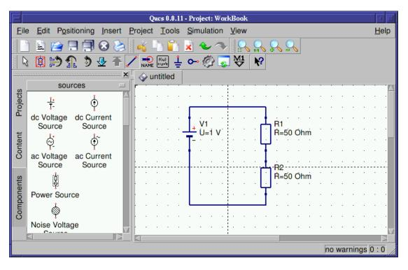
Figure 7: Components of the voltage divider appropriately wired
