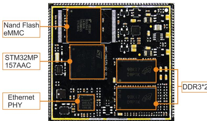
Figure 1-6 MYC-YA157C CPU Module
