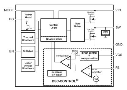
Figure 2. Functional Block Diagram (Adjustable Output Voltage Version)
