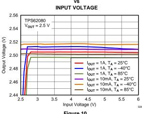
**OUTPUT VOLTAGE INPUT VOLTAGE**
