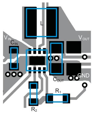
Figure 32. PCB Layout Suggestion
