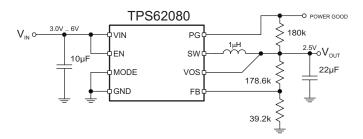
Figure 35. 2.5V Output Voltage Application (TPS62080)
