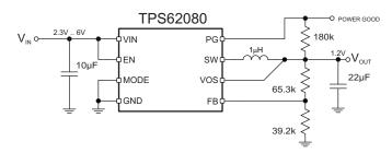
Figure 34. 1.2V Output Voltage Application (TPS62080)
