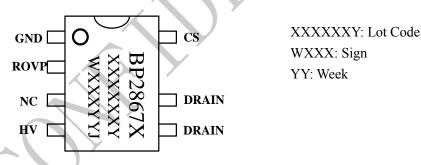
Figure 2. Pin configuration
