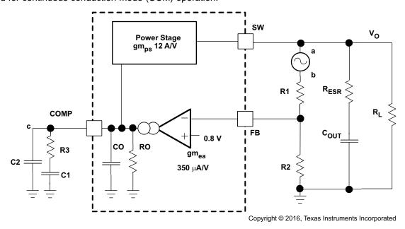
Figure 29. Small Signal Model For Loop Response
