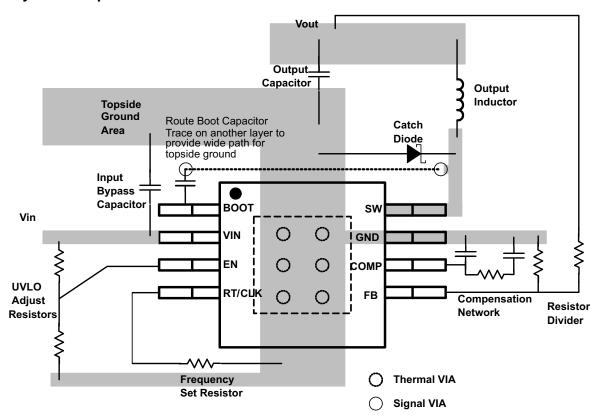
Figure 53. PCB Layout Example
