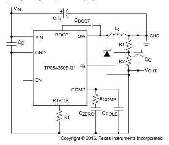
Figure 51. TPS54360B-Q1 Inverting Power Supply
