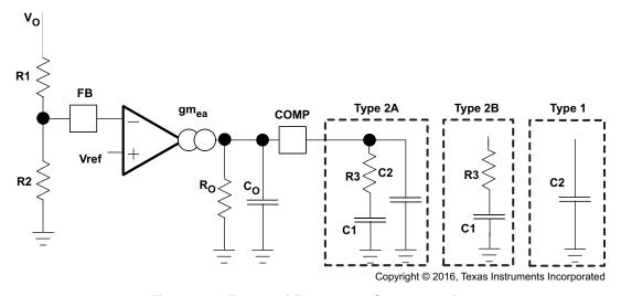
Figure 31. Types of Frequency Compensation
