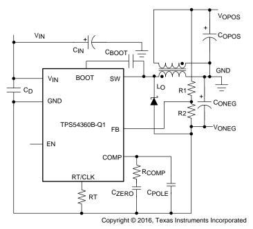
Figure 52. TPS54360B-Q1 Split Rail Power Supply
