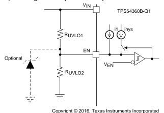
Figure 22. Adjustable Undervoltage Lockout (UVLO)
