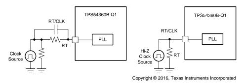
Figure 25. Synchronizing to a System Clock
